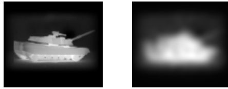
Figure 23: High-resolution picture of object (at left) and magnified LWIR diffraction limited image (at right) of the target at 10 km through a 15 cm aperture. (Note: 70x over-sampling needed for simulation; displayed here at 10% scale.)
