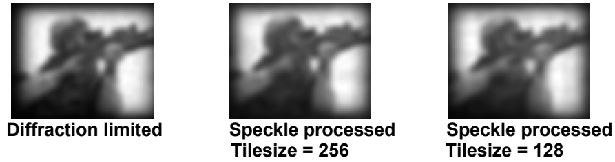
Figure 4: Simulated imagery and results for MWIR, Cn2 = 2e-13 , range = 2 km, horizontal path.
