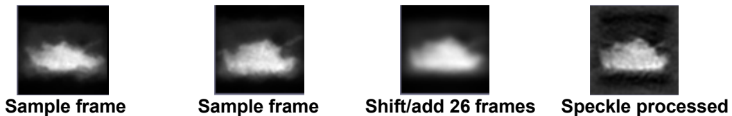
Figure 13: Simulated imagery and results for MWIR, Cn2 = 7e-14, Range = 10 km, horizontal path.
