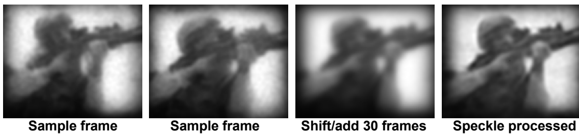
Figure 17: Simulated imagery and results for visible wavelength, C_n2 = 1e-15 , Range = 10 km, horizontal path.
