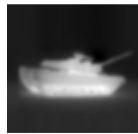
Figure 11: Diffraction limited images for a telescope diameter of 15 cm. Image is roughly 8.5 meters on a side.
