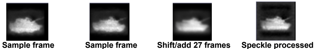
Figure 12: Simulated imagery and results for MWIR, Cn2 = 3e-14, Range = 10 km, horizontal path.
