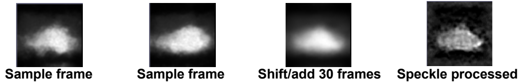
Figure 15: Simulated imagery and results for MWIR, Cn2 = 2e-13 , Range = 10 km, horizontal path.
