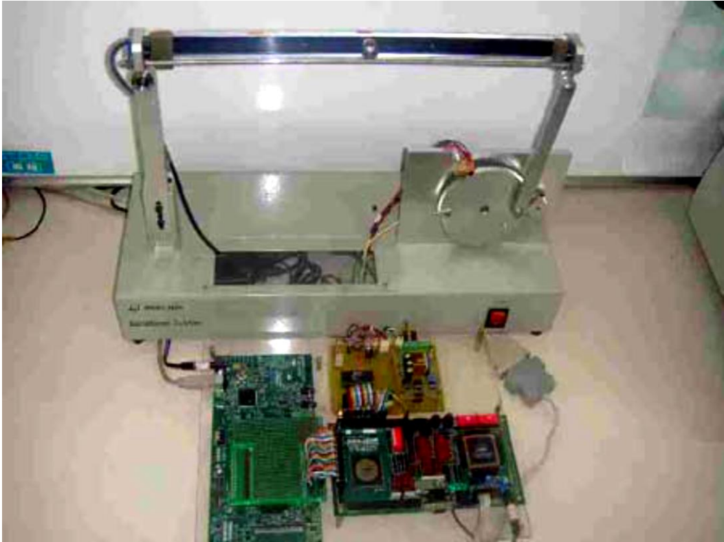
Fig 3.9: (a) The BD of the implemented digital control system and (b) the plant model used with DSP and FPGA boards (taken from [88])
