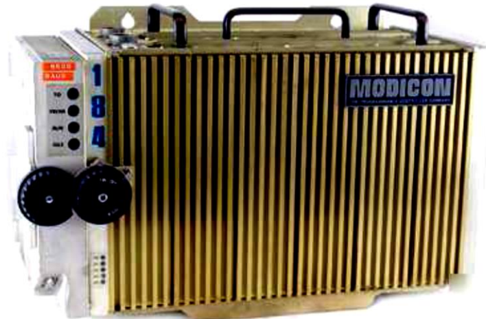
Fig 1.16 (a): The first PLC in history, Allen Bradley's the Bulletin 1774 and (b) the first Modicon PLC (taken from [1])
