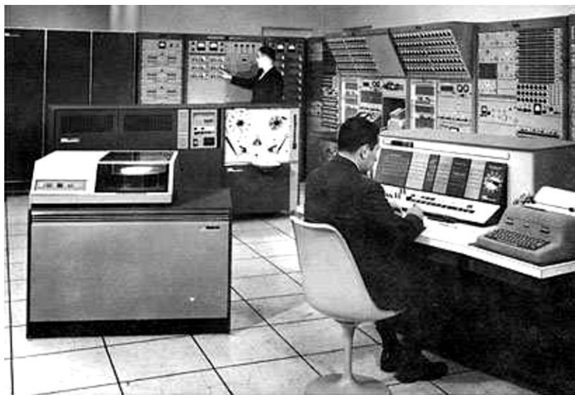
Fig 1.11: The use of digital computers in control rooms as indications and operation while the actual control was analog circuitry (taken from [1])
