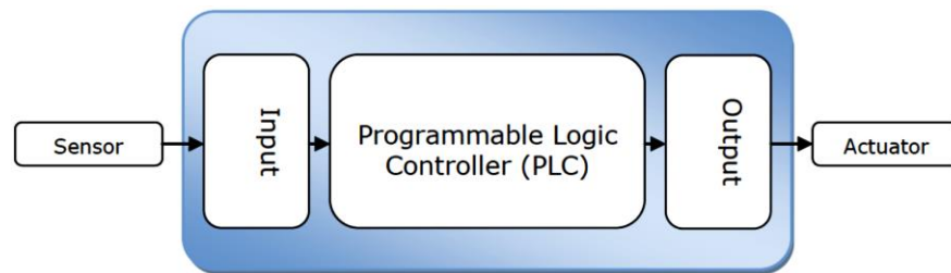
Fig 2.36: A simplified BD of PLCs architectural I/O advantage (taken from [61])
