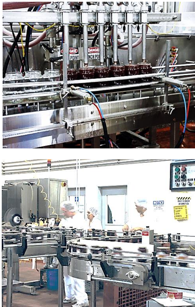
Fig 1.4: Discrete manufacturing (a) packing and (b) assembling processes
