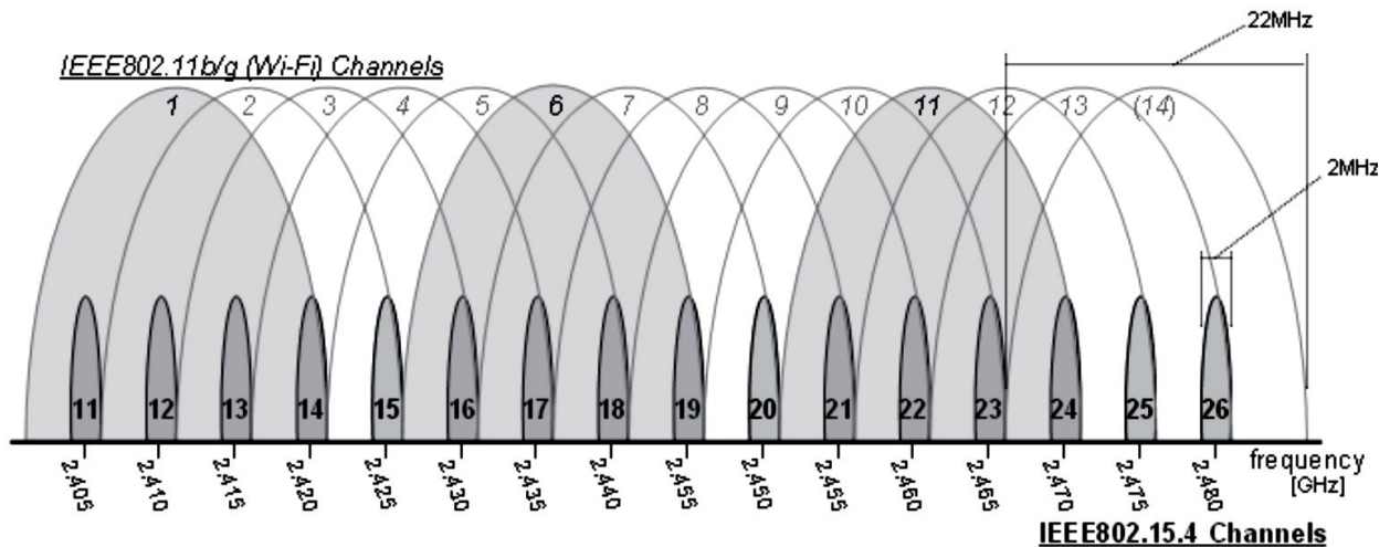
Fig 1.44: Wi-Fi as a backbone to 2.4GHz WSN channels (taken from [34])
