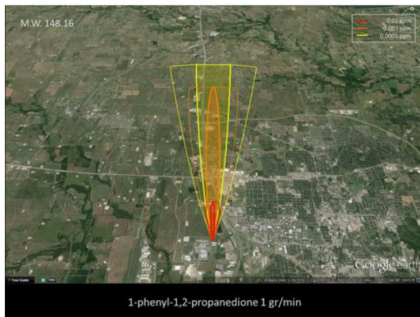
Figure 3.11. Thread zones of organic compounds at a pollutant rate of 1 gr/min.
