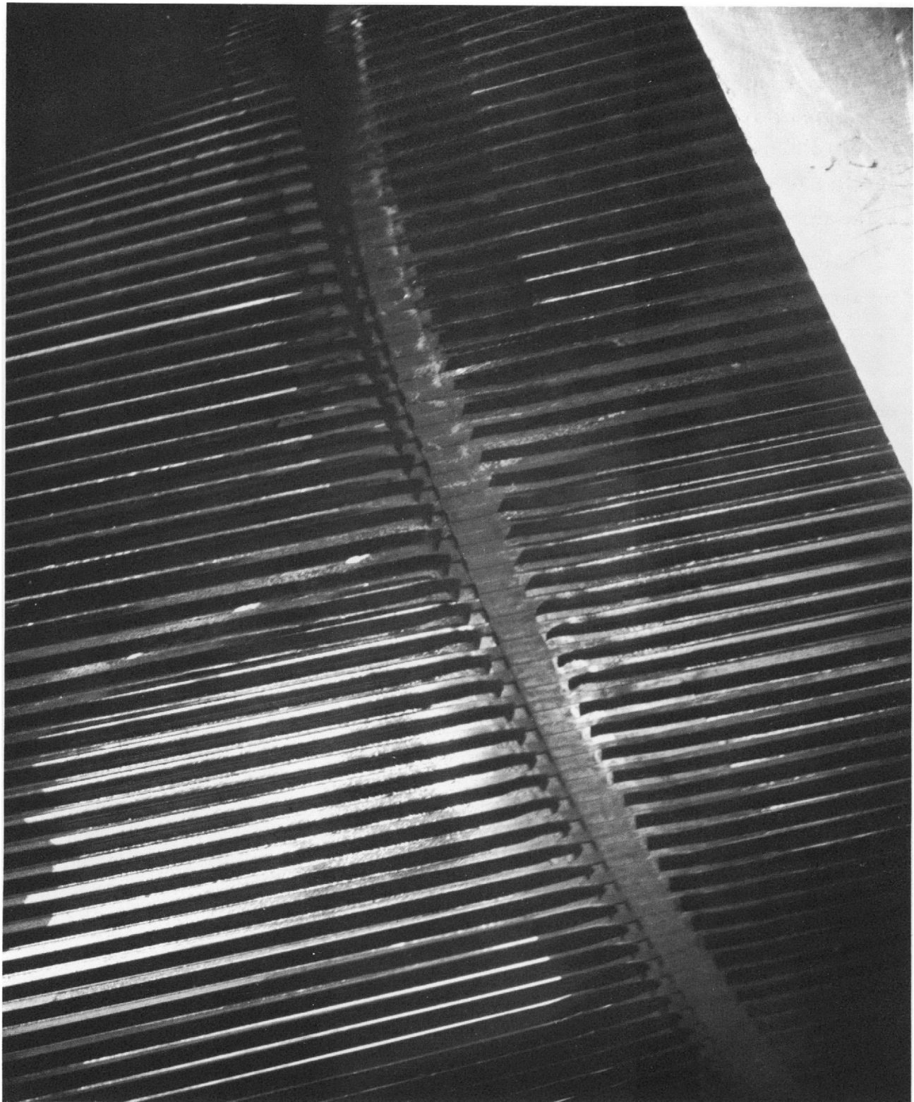
Figure 21. Close-up of the Junction Region Between Two of the Outer Fuel Cylinders
