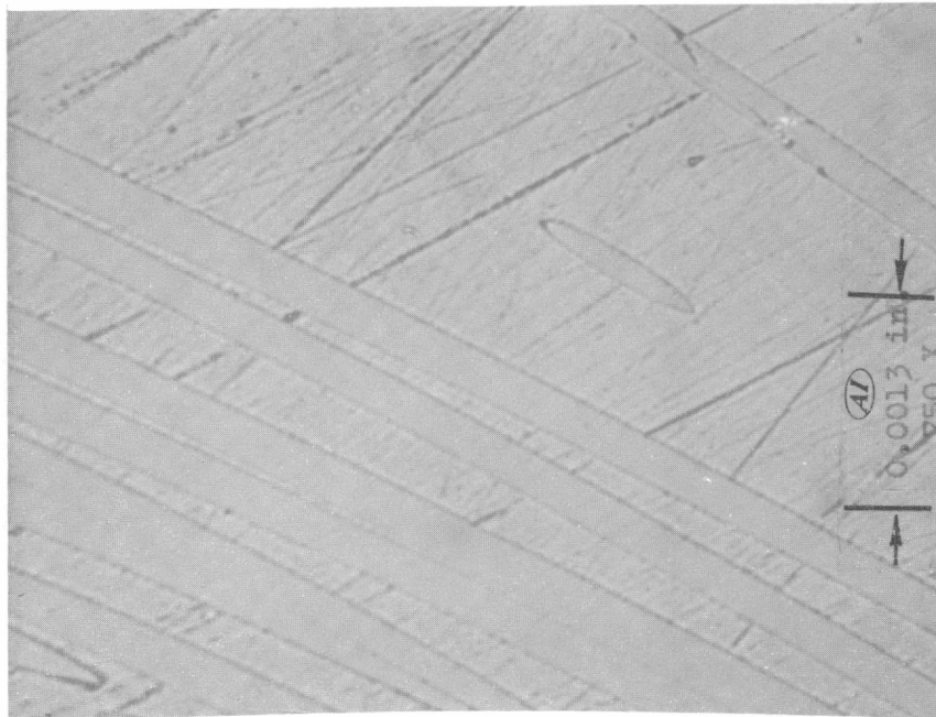
Figure 28. Longitudinal Section of Used Glass Fibers
