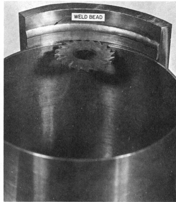
Figure 14. Section Showing Typical Cut Made in Simulated Process Tube
