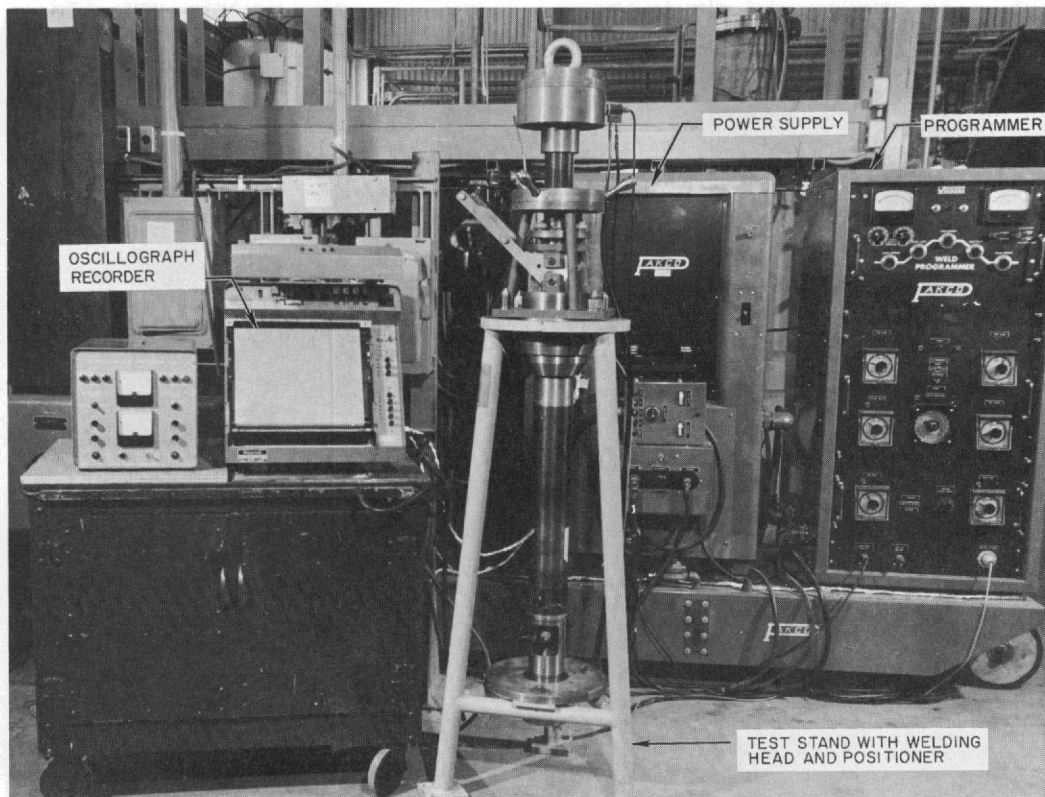
Figure 10. Welding Test Setup with Automatic Programming Equipment
