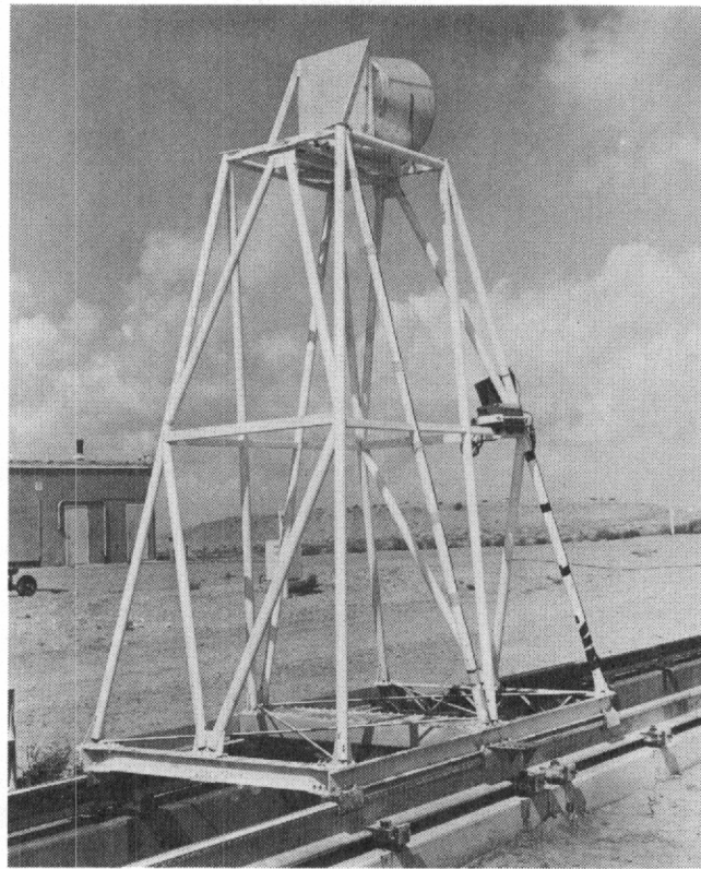
Figure 78. Test setup for sled tests of an aluminum simulated version of the parachute compartment
