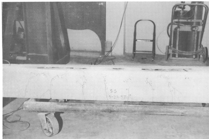
Typical Balanced Failure — f_{se} = 0 \text{ psi} , r = 4.16 \%
