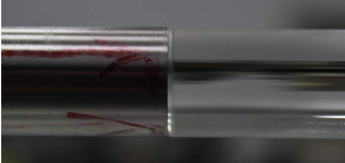
Figure 0.4 Alignment between incident bar and glass sample
