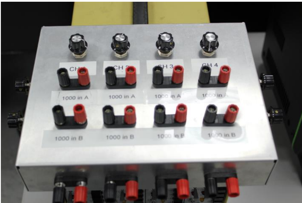
Figure 0.4 Image of a Wheatstone bridge
