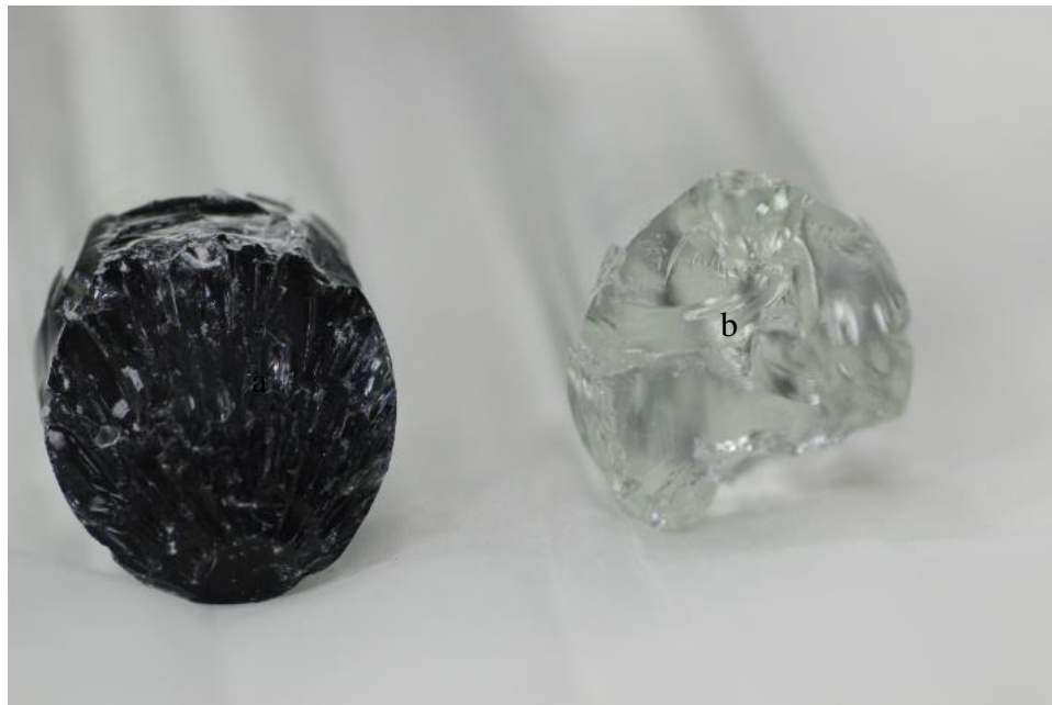
Figure 0.7 Figure showing (a) tensile failure striations and (b) random failure
