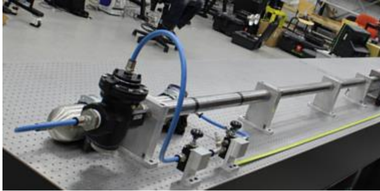
Figure 0.1 Barrel mounting and firing setup
