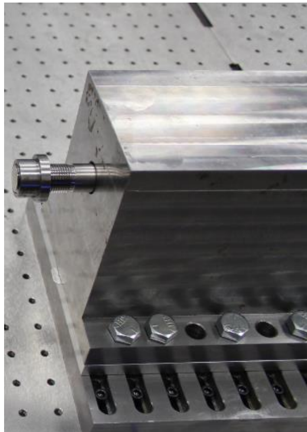
Figure 0.6 Momentum trap with incident bar (and attached flange) protruding
