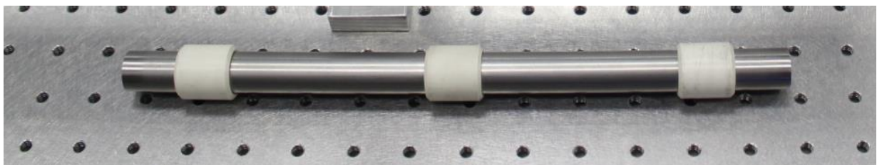
Figure 0.2 Striker with attached sabots
