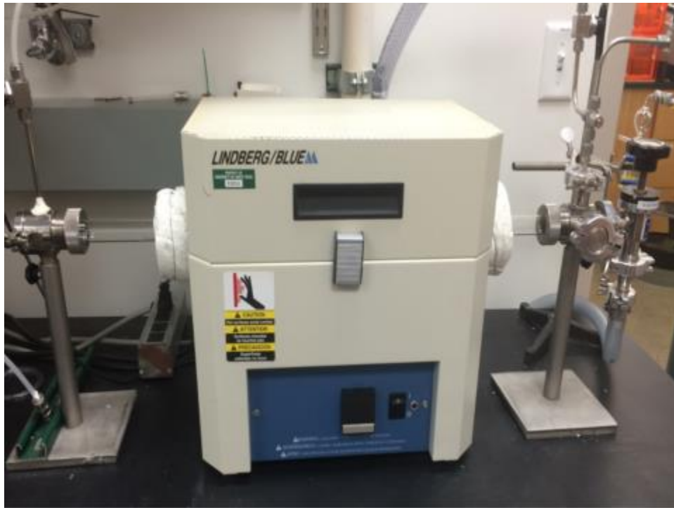
Figure 1.6: CVD system in Dr. Chyan's laboratory.
