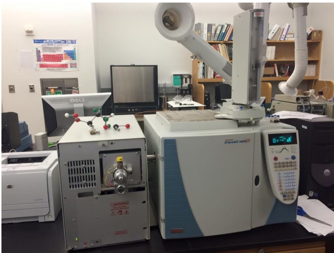
Figure 1.19: Finnegan TraceGC ultra Trace DSQ Mass Spectrometer used in Cu/Al bimetallic corrosion analysis.
