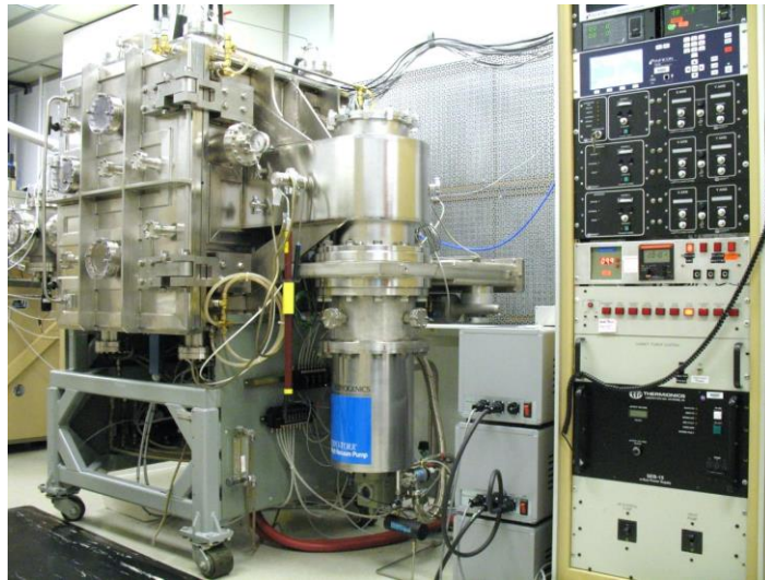
Fig. 3.1: Photograph of the Thermionics Vacuum Products Co. Triad e-beam evaporation system with accompanying power supply and control electronics. Photograph courtesy of Ron Goeke from Sandia National Laboratories.
