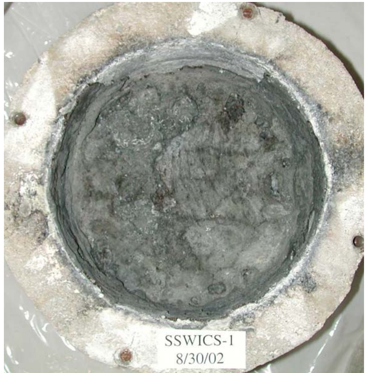
Figure 7.1 Solidified corium within MgO liner (top view).
