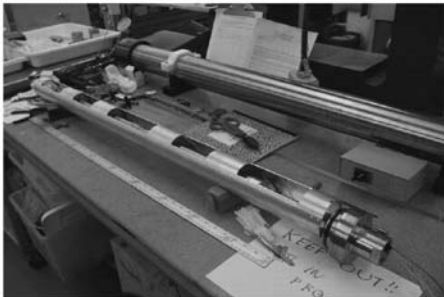
(c) Gas confining cell (top right) and a suspension cage (front) housing the sample-bar assembly
