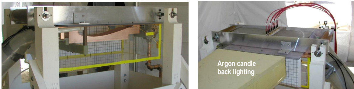
Figure 4. (left) Photo of LLNL's flat-plate FCG set up for first test. (right) Photo of other side with foam box containing argon that is explosively shocked for back illumination while imaging using high-speed rotary mirror camera.
