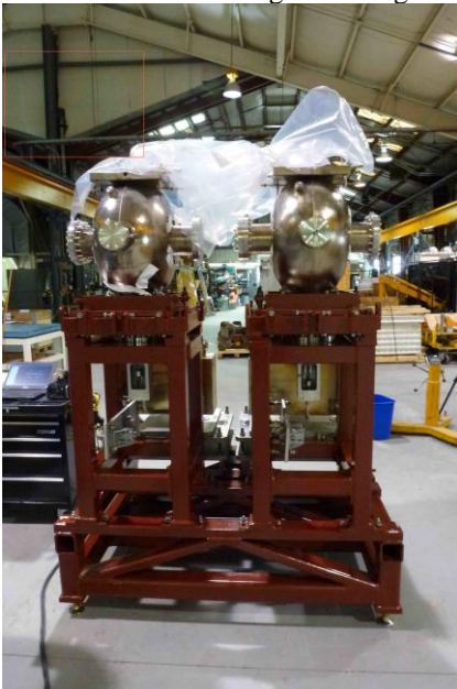
Figure 4: Two 500 MHz cavities mounted on a common support before installation into the IP2 region.
