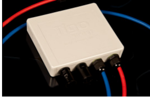
Figure 81: Redesigned Maximizer unit with reduced footprint and thickness
