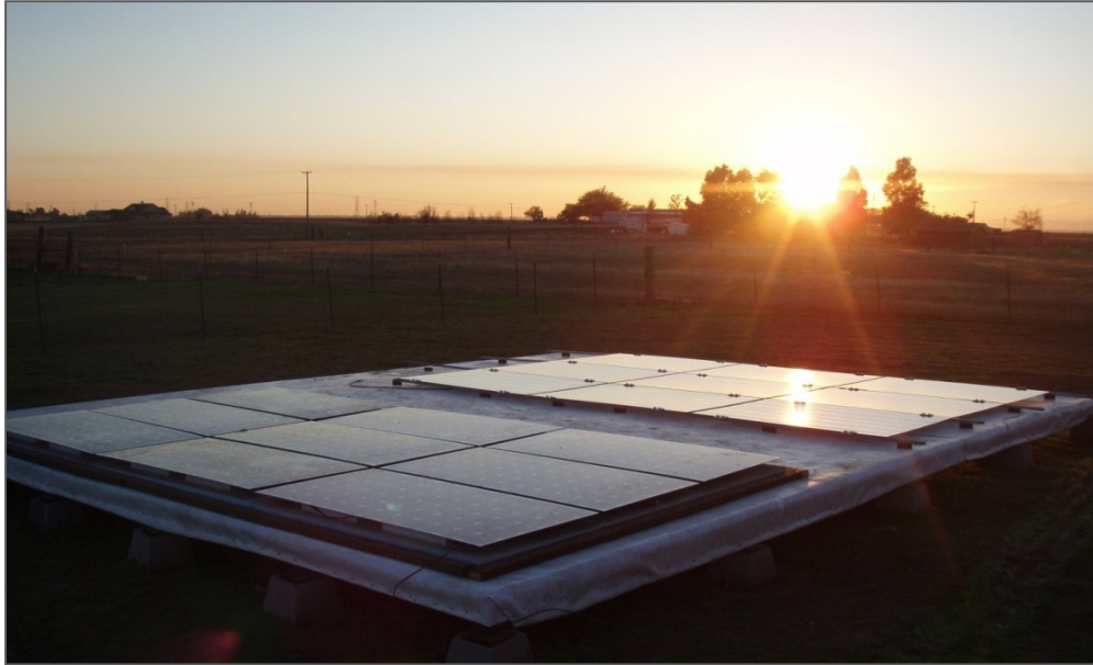
Figure 27: Unconstrained Commercial Roof Product prototypes installed at test site
