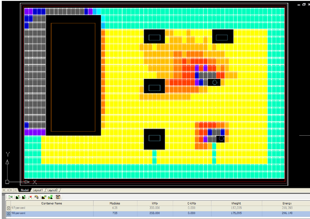
Figure 47: Sample T5 layout on a rooftop with shading obstructions and relative module energy production ranked using the PVFast color code
