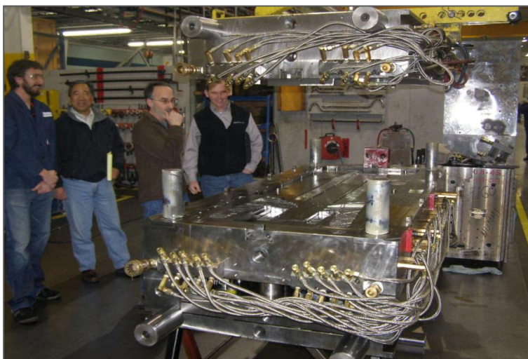
Figure 21 Production mold for T5 frame components at supplier facility in California
