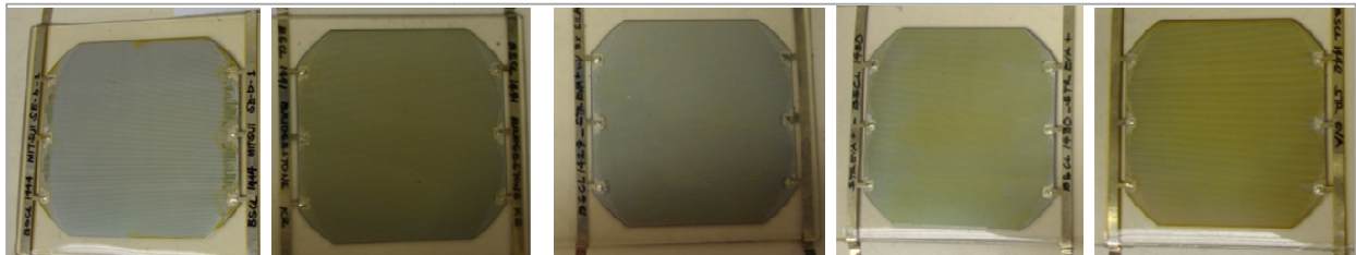
Figure 11: Examples of accelerated browning on a variety of bifacial backsheet and encapsulant candidates
