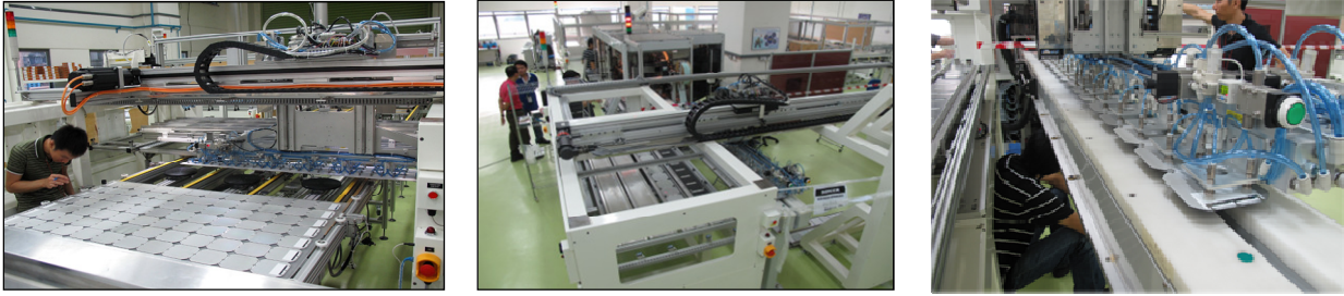
Figure 37: Photos of stringer integrated into auto-up system during process qualification at vendor
