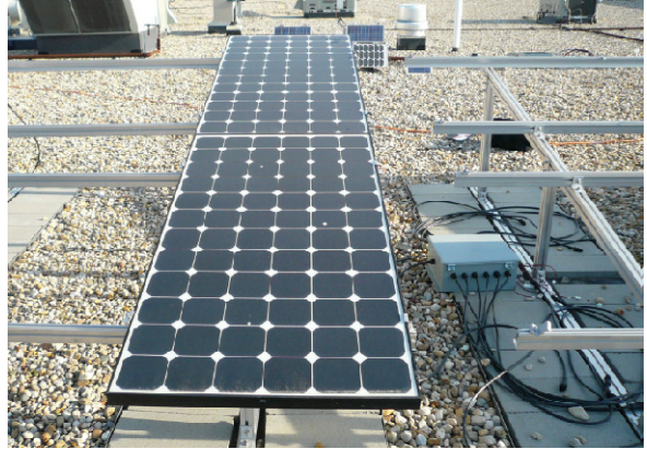
Figure 75: Setup for outdoor testing of SP225 PV modules
