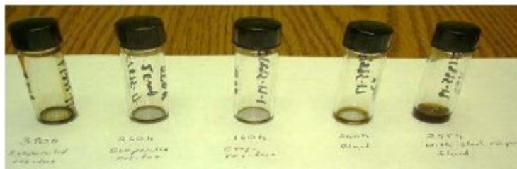
Figure 16. Photograph of evaporated cyclopentene. Samples after 390, 260, and 160 hours at 300 °C (left 3 vials) and non-evaporated cyclopentene after 260 and 255 hours (right 2 vials).
