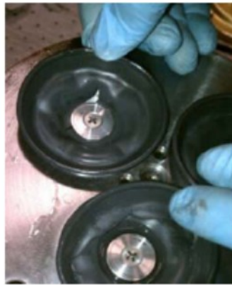
Figure 27. Ripped Viton diaphragms showing that Viton is not compatible with the new fluid.
