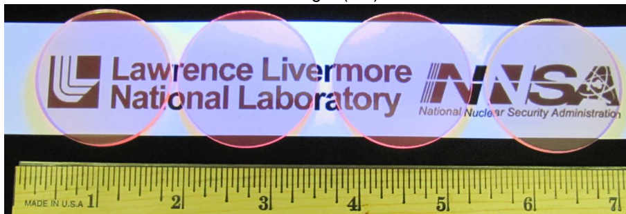
Figure 7. (top) Beta radioluminescence spectra of transparent ceramic GLO(Eu) compared with CdWO 4 and CsI(Tl), spectra may be directly compared and represent their absolute light yields. (bottom) A photograph of four 4.2 cm diameter by 0.2 cm thick GLO(Eu) radiography ceramics in room lights and under weak UV illumination, displaying the orange Eu 3+ emission.
