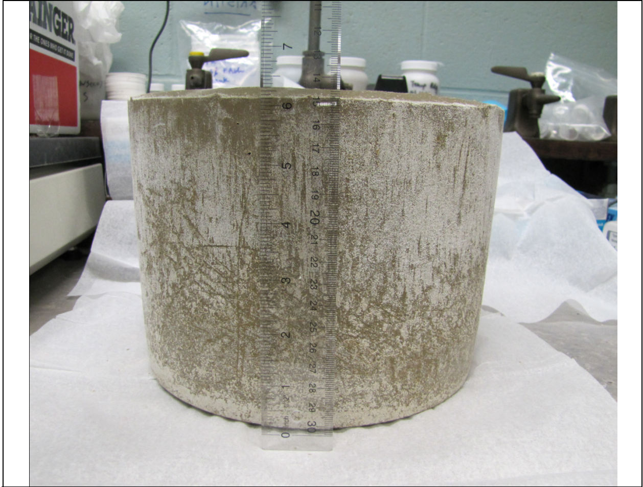
Figure 8-3. Waste form (2 gal) after removal from the mold. Notice slight expansion on the top surface
