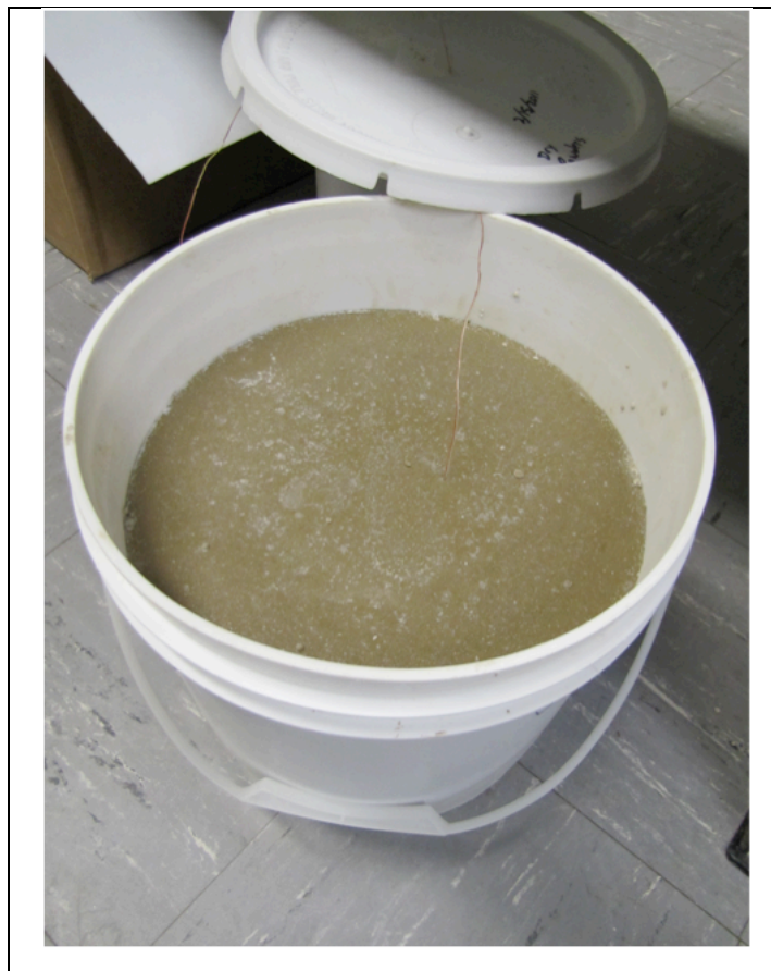
Figure 8-2. Waste form (2 gal) after 3 days of curing
