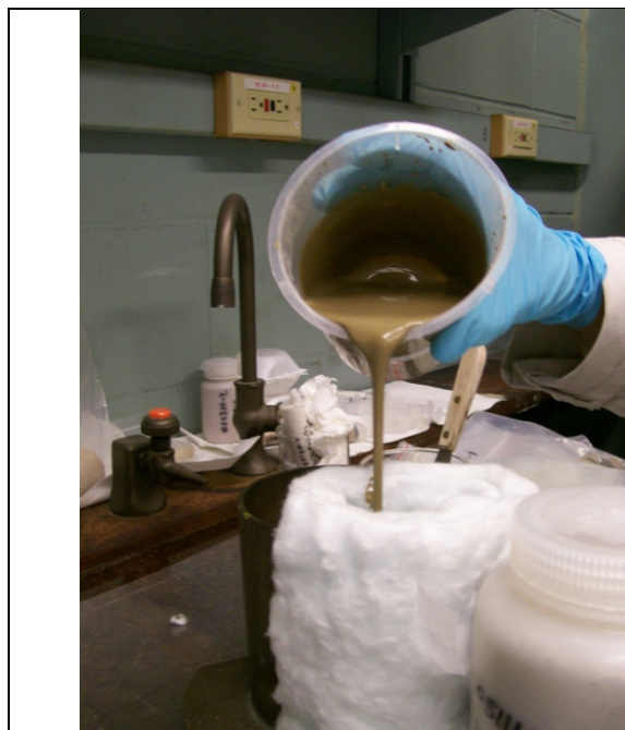
Figure 3-3. Slurry of Ceramicrete mix with Class C fly ash and 20 wt.% baseline waste simulant
