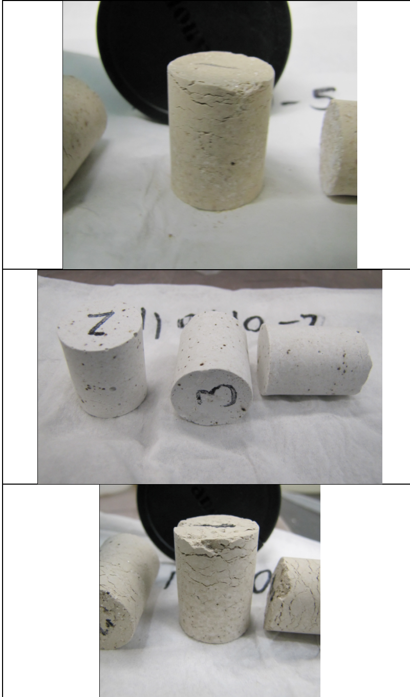
Figure 6-3. Waste forms with 15 wt.% waste cluster 1 waste simulant loading after 90-day ANS 16.1 test: (top) 45 wt.% Class C fly ash, (middle) 45 wt. \text{CaSiO}_3 , and (bottom) 35 wt.% Class C fly ash + 10 wt.% slag
