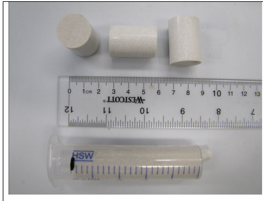
Figure 4-2. As-fabricated waste form for 45 wt.% \text{CaSiO}_3 and 20 wt.% baseline waste simulant
