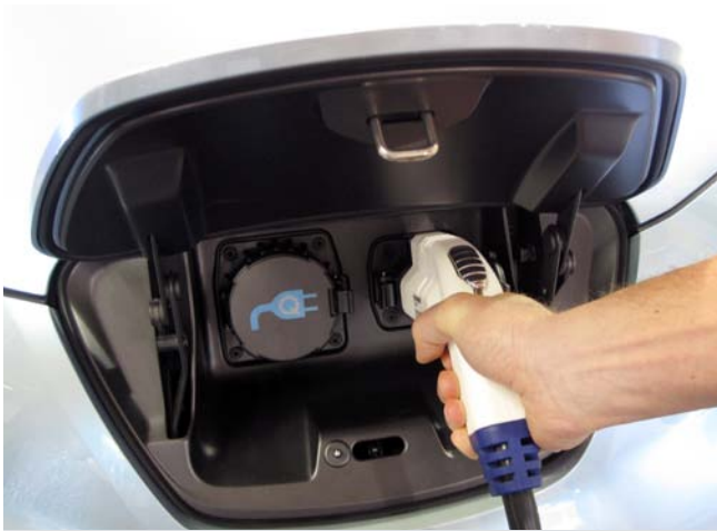
Figure 4. The standard SAE J1772 EVSE connector fits into the standard SAE J1772 receptacle. Photo by Andrew Hudgins, NREL/PIX17634
