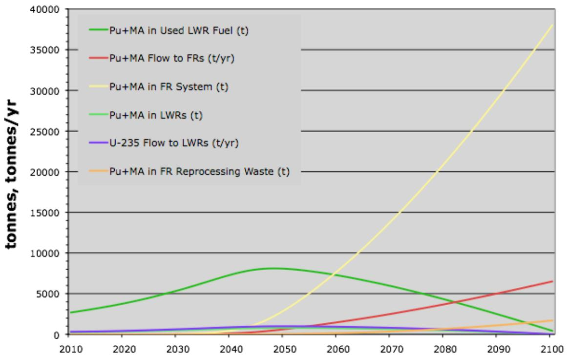
Figure 4a. Power production and stocks and flows of Pu+MA and  $^{235}\text{U}$  for CR = 1.21,  $\tau_F = 2$  years.
