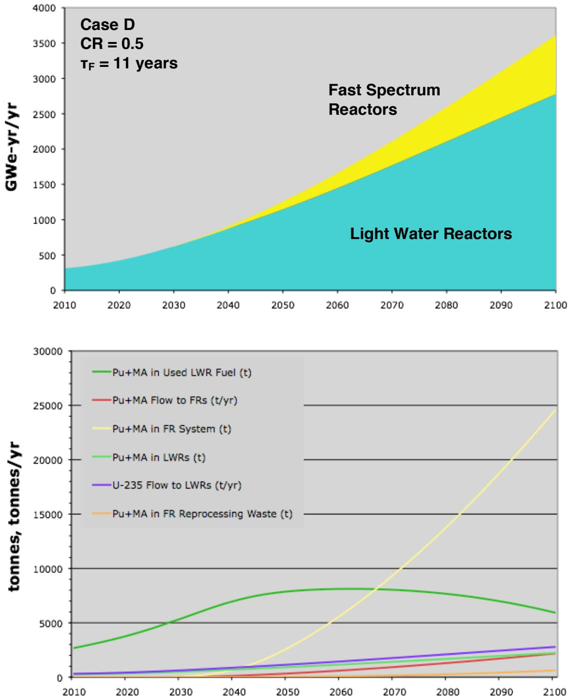
Figure 4d. Power production and stocks and flows of Pu+MA and  $^{235}\text{U}$  for CR = 0.5,  $\tau_F = 11$  years.
