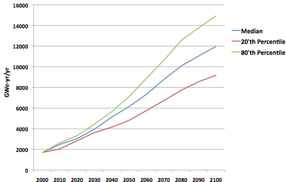
Figure 1. Electrical power production from EMF 22 models. “GWe-yr/yr” is used to indicate electrical power production, as opposed to production capacity, often denoted “GWe”.
