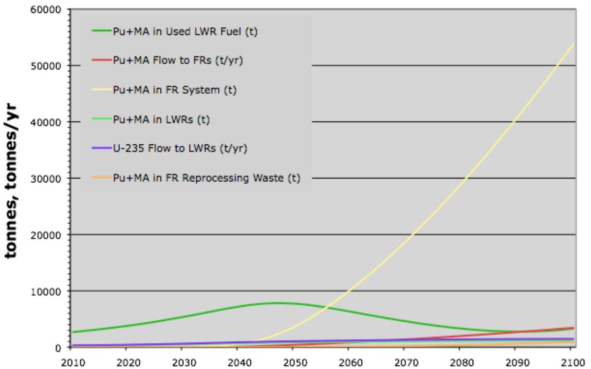
Figure 4b. Power production and stocks and flows of Pu+MA and  $^{235}\text{U}$  for CR = 1.5,  $\tau_F = 11$  years.
