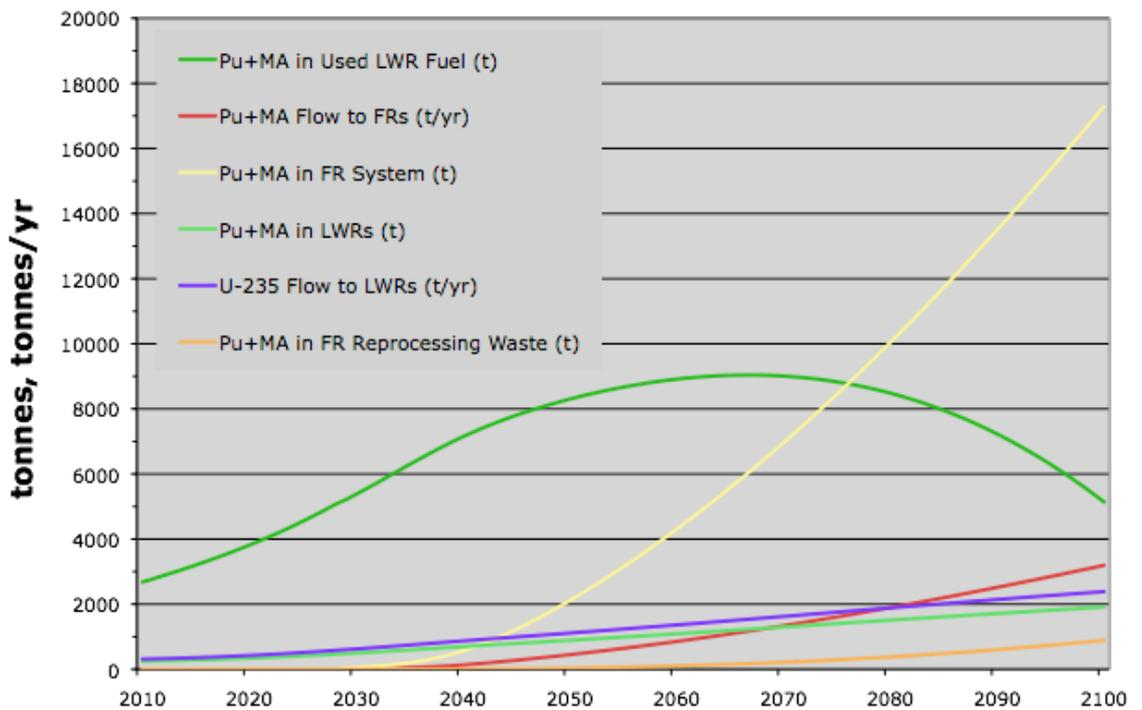
Figure 4c. Power production and stocks and flows of Pu+MA and  $^{235}\text{U}$  for CR = 0.5,  $\tau_F = 2$  years.
