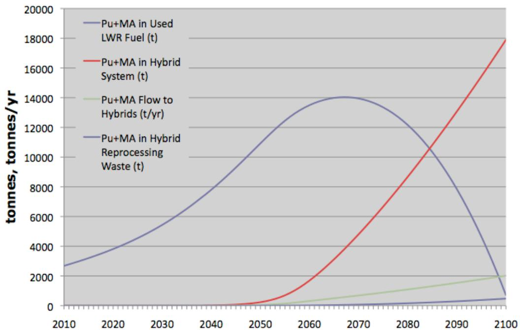
Figure 6. Stocks and flows of Pu+MA in fission-fusion hybrid case.
