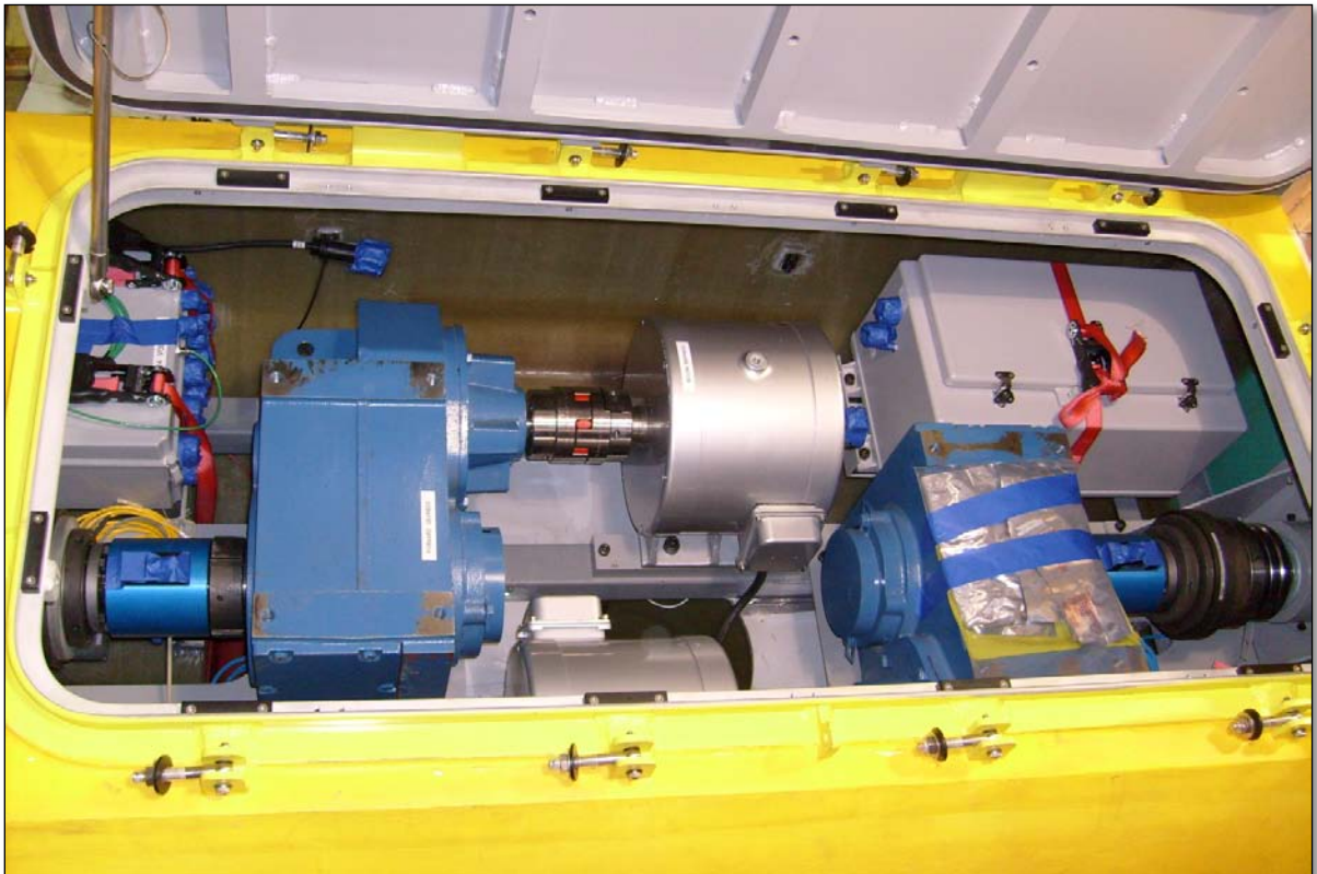
Figure 3 - Dual PTOs installed in the SeaRay beneath the main access hatch.
