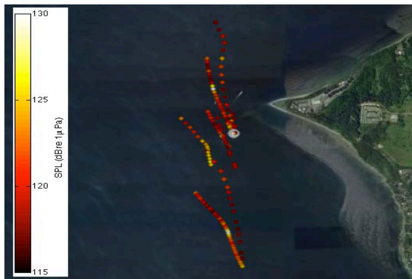
Figure 2. Spatial distribution of recorded broad-band SPLs (20 Hz - 20 kHz in dB re. 1 uPa). The white circle at the center indicates the location of the SeaRay near West Point (Puget Sound, WA), and the region shown is 3 x 3 km.
