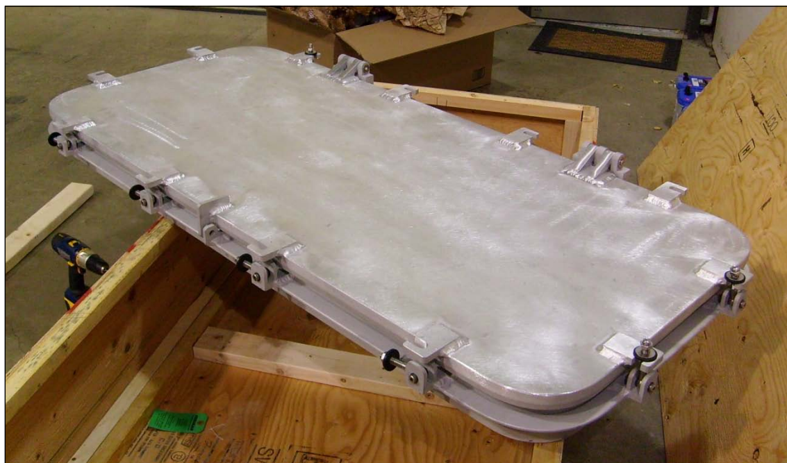
Figure 8 - Watertight aluminum hatch manufactured by Freeman Marine, Gold Beach, OR.
