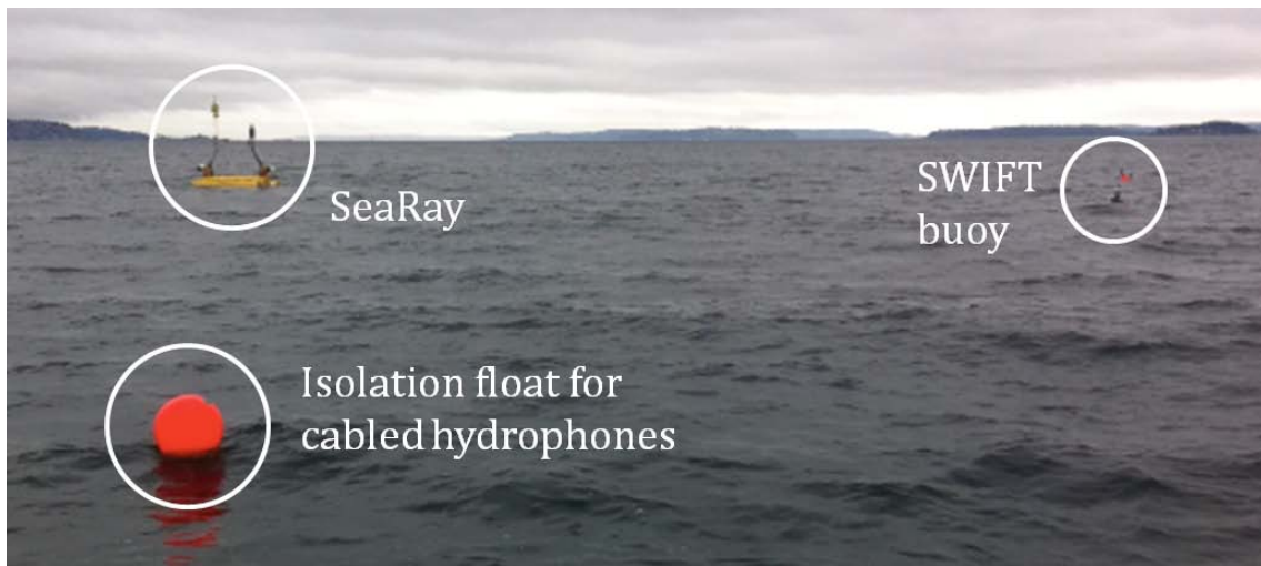
Figure 1. SeaRay (upper left), cabled hydrophone isolator float (lower left), and autonomous drifting hydrophone (upper right).
