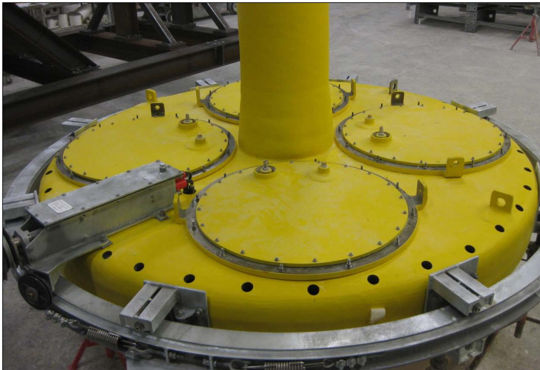
Figure 49 – SeaRay damper tank showing the yaw control system and yaw drive motor.
