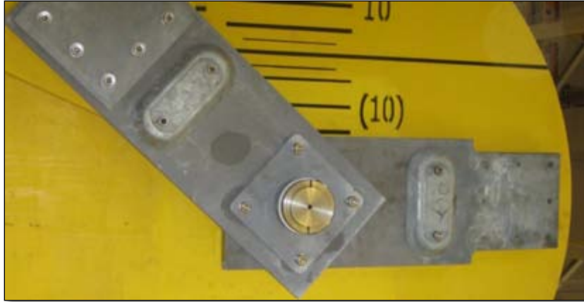
Figure 9 - Float arms connected to PTO shaft with zinc anodes and depth gauge on nacelle.
