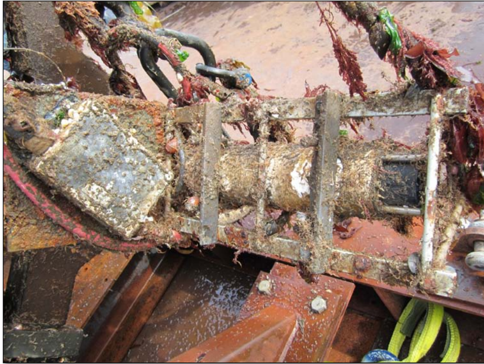
Figure 47 – Typical biofouling on acoustic modem and mooring hardware.
