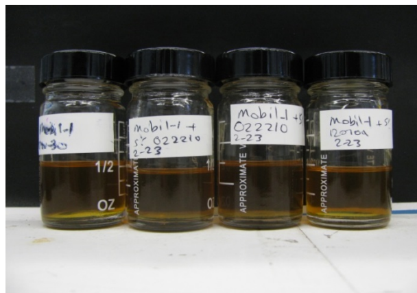
Figure 11. Blending of a fully formulated synthetic oil with 5% of milled boric acid in canola oil, modified canola oil, and soybean oil. The result was a clear product that was very stable for a long period of time.
