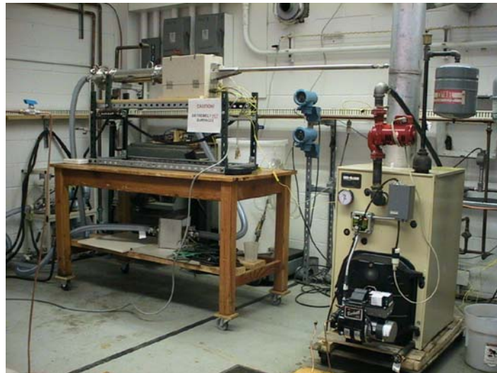
Figure 2. Cast iron boiler and PM 2.5 Dilution Tunnel Sampler
