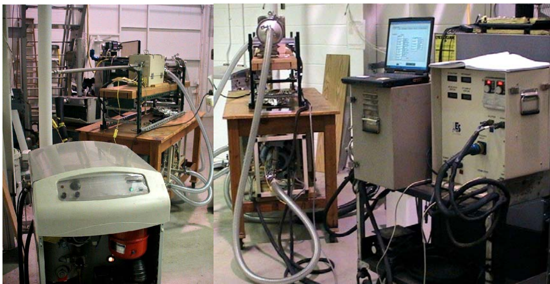
Figure 8. Oil-fired condensing steel boiler during PM 2.5 dilution tunnel testing
