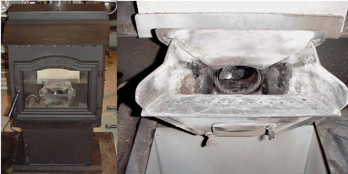
Figure 14. Pellet stove, side feed burner, open burner grate, and manual gel ignition
