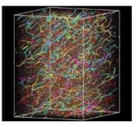
Fig. 7. Simulated dislocation-defect structure after plastic deformation in Fe-Cr-Ni steel.
