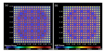
Fig. 1. Translation of Denovo output to AMP: (a) Cross section of fuel assembly showing Denovo-calculated power distribution. (b) The same data represented in the AMP mesh
