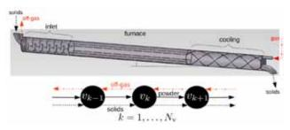
Fig. 4. Voloxidization calciner with network representation of flows and holdup.
