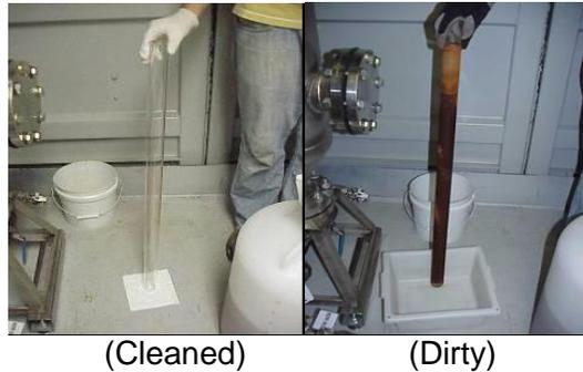
**Figure 2. Fouling of the UV Light Apparatus**
