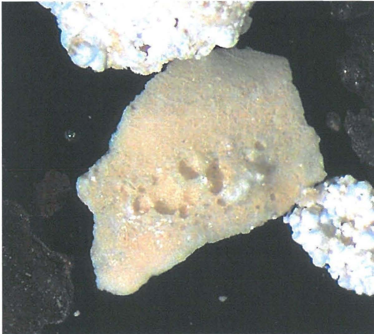
Figure 5 Aggregate of Salt Crystals showing Glassy and Vesicular Morphology from Sample 2AY-12-ANU-3A.
