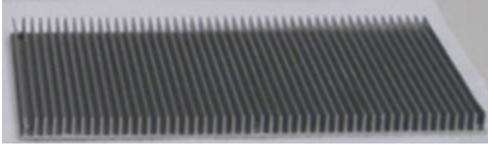
Figure 24: Linear fin heat sink 125 mm in width by 72 mm in length by 5.7 mm in height with a base thickness of 0.8 mm and having 50 fins, each with a height of 4.9 mm, width of 0.5 mm and a pitch of 2.5 mm that is CNC machined from aluminum with a conductivity of 160 W/mK.
