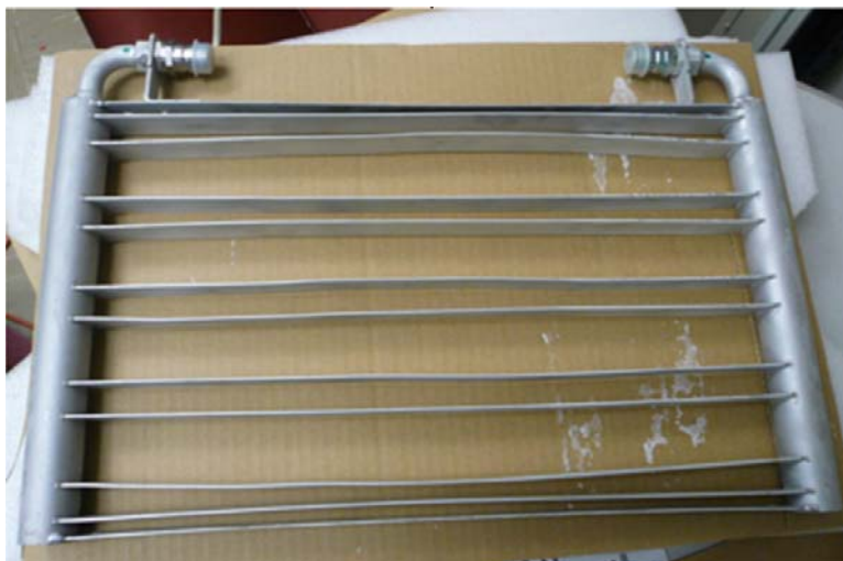
Figure 34: Photograph of a modified finless heat exchanger, intended to serve as a thermal backplane. The finless heat exchanger was made by Modine. The 12 multiport heat exchangers run horizontally in this view. Thermal modules will be clamped to these surfaces for cooling of on-board devices.
