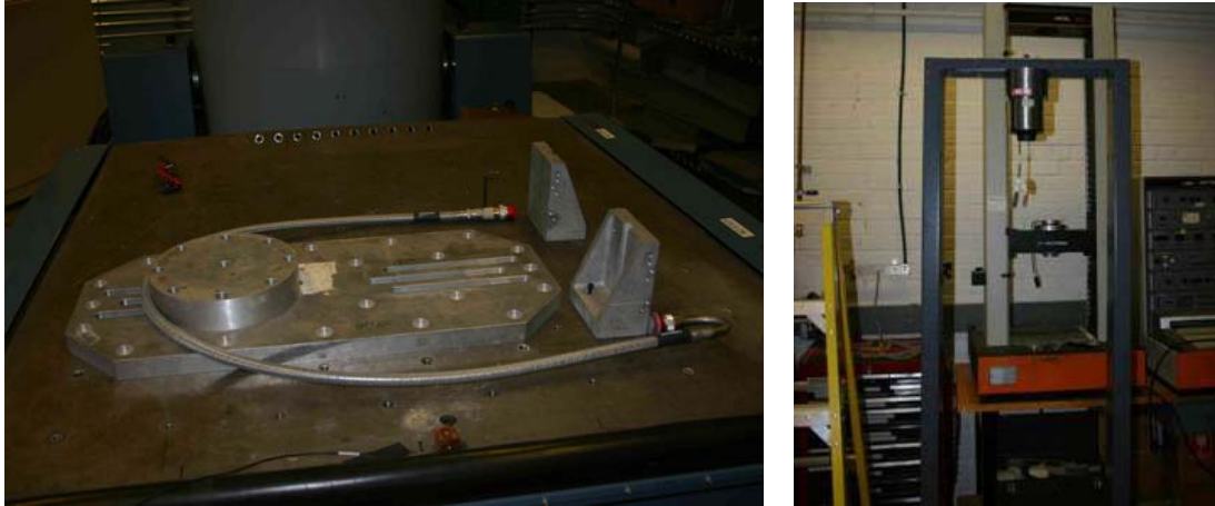
Figure 66: Test fixtures developed for evaluating the mechanical integrity of the non-conductive hose assembly: (left) random vibration test fixture; and (right) drop test fixture.
