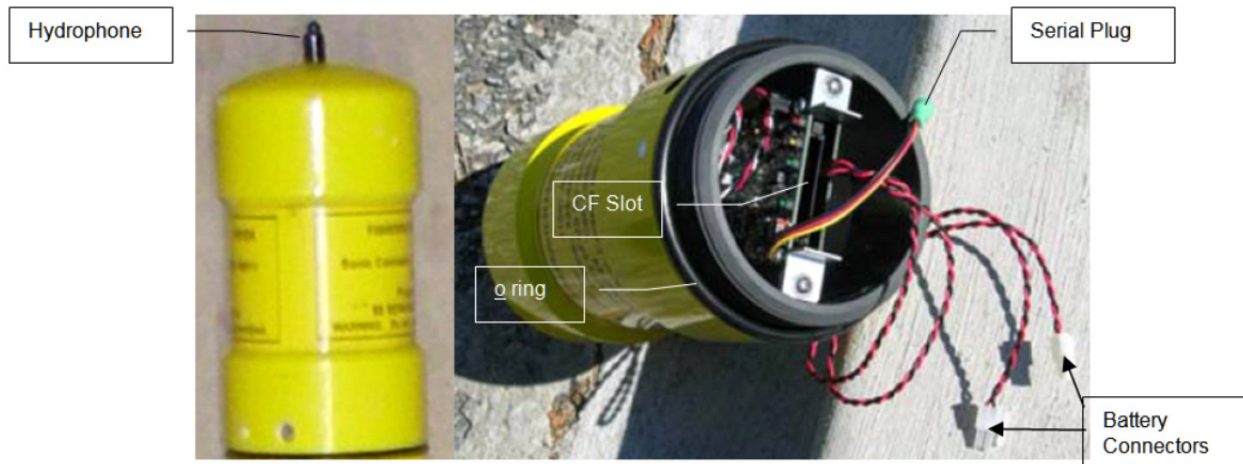
Figure 3.11. Side (left) and bottom (right) views of the top of an autonomous node.
