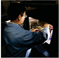
The High Energy Battery Test Facility at the Energy Systems Laboratory houses over 650 battery test channels, environmental chambers, a shake table, and related battery testing equipment and test vehicle platforms for evaluating new battery technologies under development for automotive applications.
