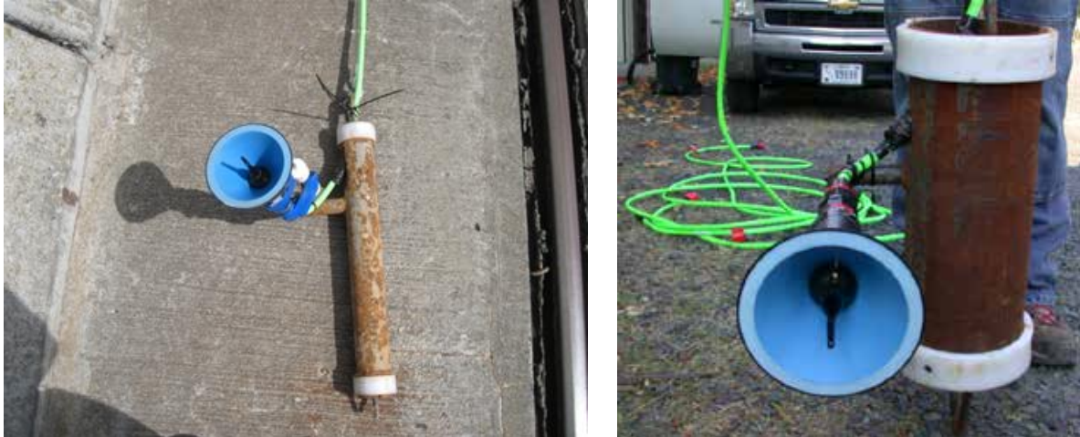
Figure 2.8. Trolleys Used to Deploy Hydrophones at B1 and B2 (left) and the Spillway (right). The photos show 4-in.- (left) and 8-in.- (right) diameter trolleys for slotted pipes. Each trolley had a steel arm to support a hydrophone that was surrounded by a plastic cone lined with anechoic material to prevent sound reception from a downstream direction. The white polyvinyl chloride object immediately to the right of the hydrophone baffle in the left picture is a reference beacon that was attached to four or five trolleys at each dam structure (B1, spillway, and B2).
