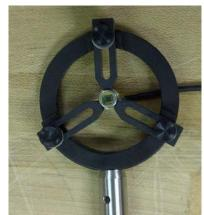
*Figure 4: Pyroelectric single cell detector mounted on a holder.*
