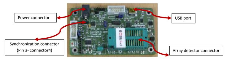
Figure 2: Sensor PCD board.
