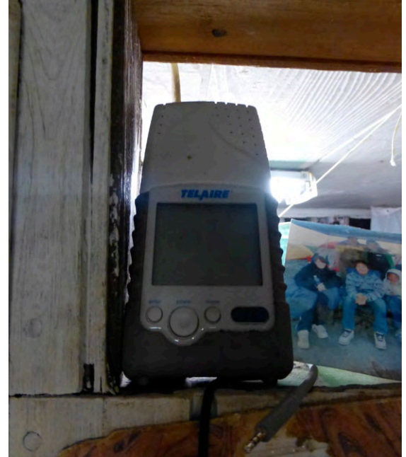
Glen Joe Sr. House. In a prior weatherization application the family was provided with a humidity monitor that beeps at them when humidity is high, and they turn the fan on to create air exchanges.
