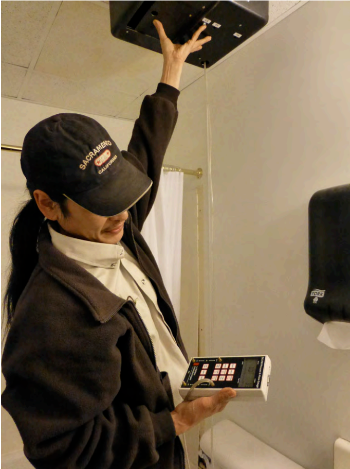
Thomas Olson performs a ventilation test at the Sea Lion Building as part of his energy assessor training.
