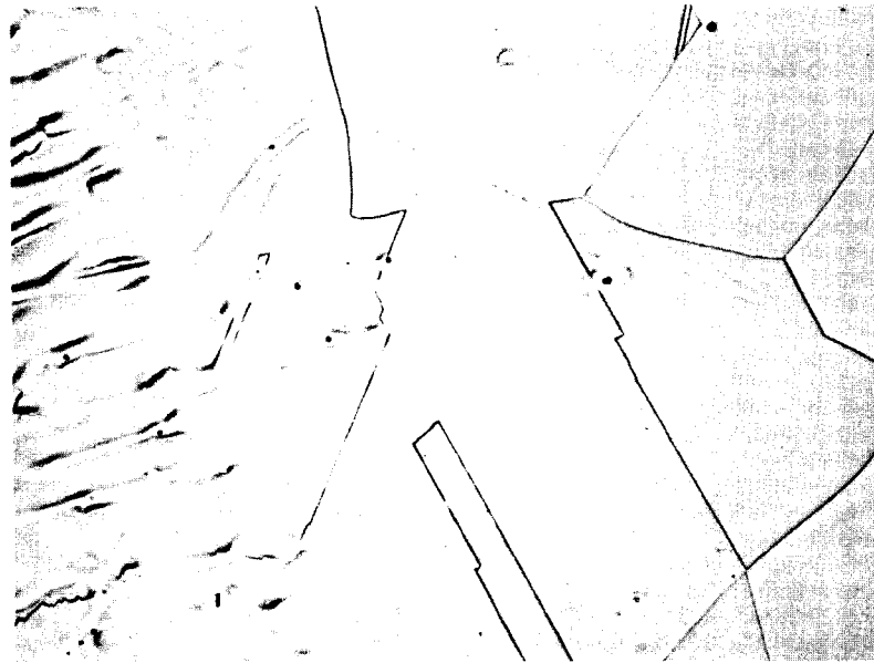
FIGURE 7.10. Stabilized Grain Structure in Type 316 SS
