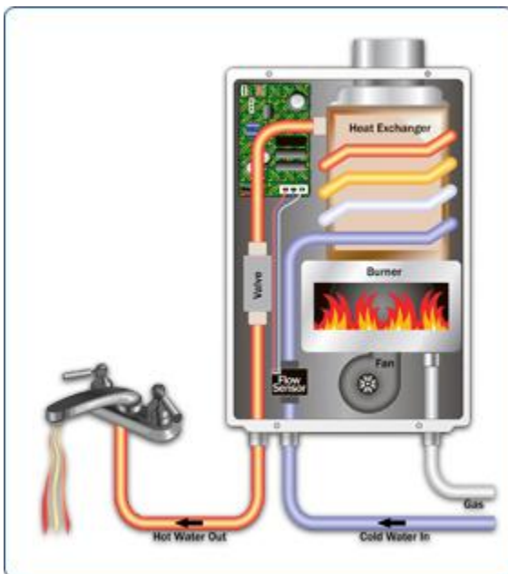
Diagram 2: A Typical Tankless Water Heater
