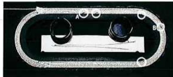
Figure 2. Coil HTS-SC08 and witness barrels and wires after reaction. Leakage spots are indicated by white circles. Spots A and B both contain large amounts of Bi and Sr, and traces of Ca and Cu, indicating that they originate from the wire cores.
