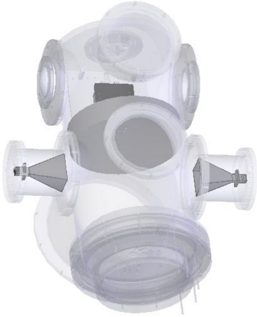
Figure 14. Depiction of chirped pulse FTMW spectrometer at UNT.
