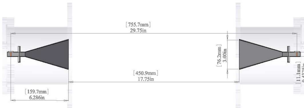
Figure 15. Depiction of the horn antennas of the chirped pulse FTMW spectrometer.
