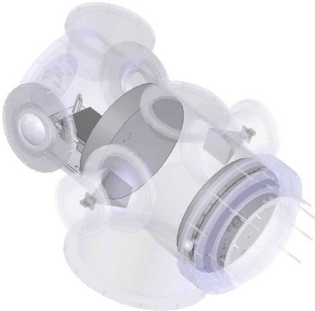
Figure 2. Representation of the Classic Balle-Flygare FTMW Spectrometer of UNT.
