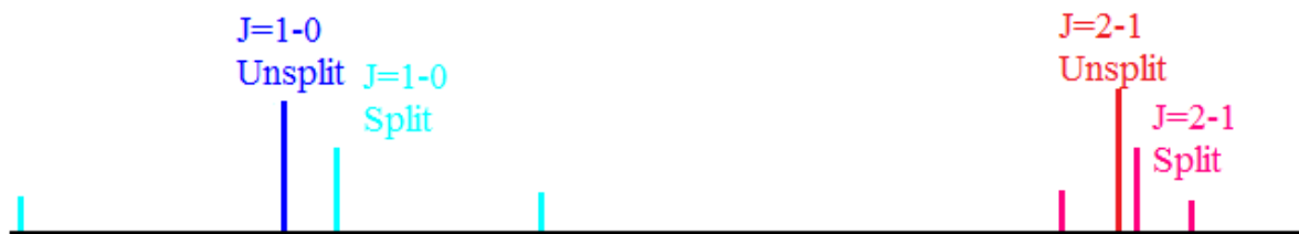
Figure 25. Depiction of the effects of nuclear quadrupole coupling (Split) on a simple spectral pattern for a linear molecule (Unsplit).
