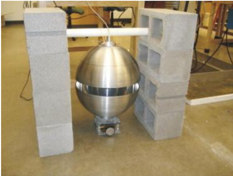
Figure 8. A photograph of preliminary testing before placing under vacuum that proved that the mirrors could be tuned to form standing waves at lower frequencies.
