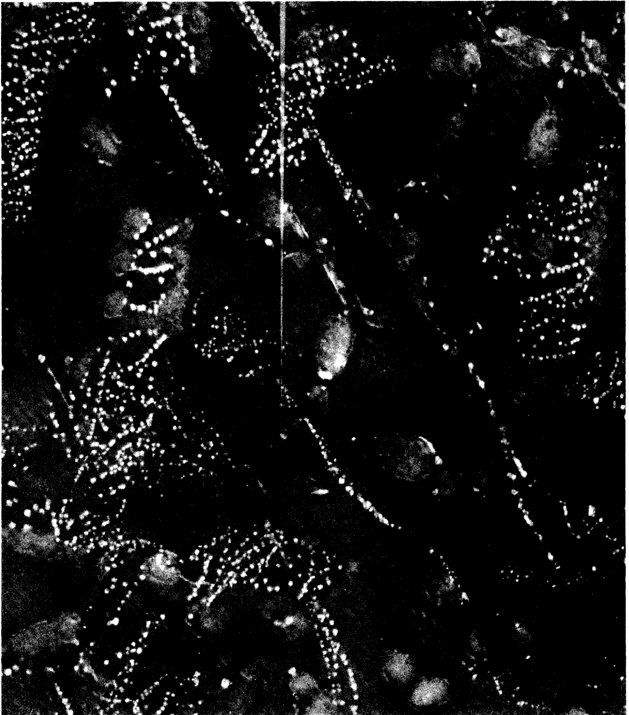
FIGURE 67. Dark Field Micrograph of Figure 9 Showing High Concentration of Finely Dispersed NbC Precipitates
