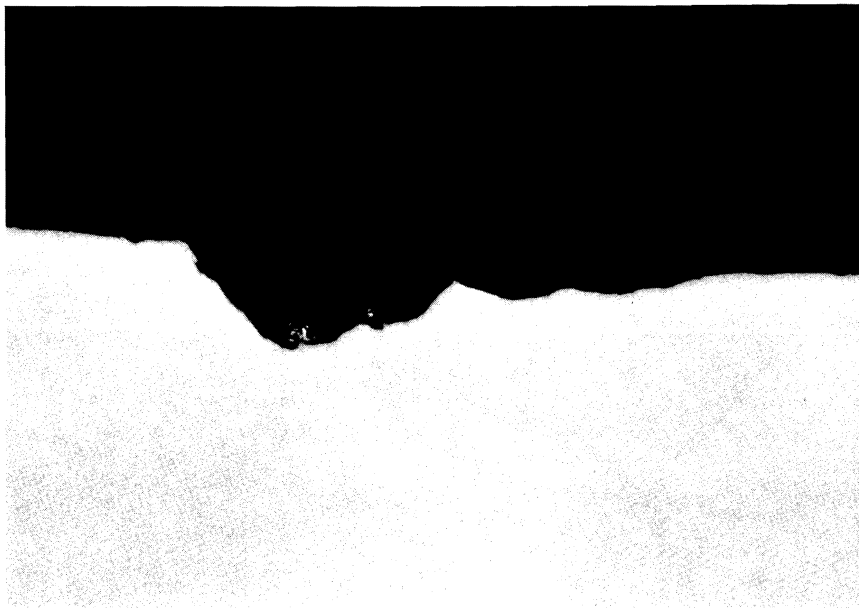
(b) Section through pit
