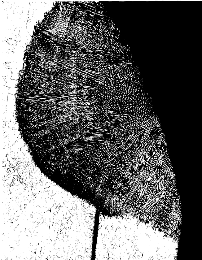
FIGURE 17. Typical Fuel Pin Closure Weld (316 SS) PNL-6,7,8
