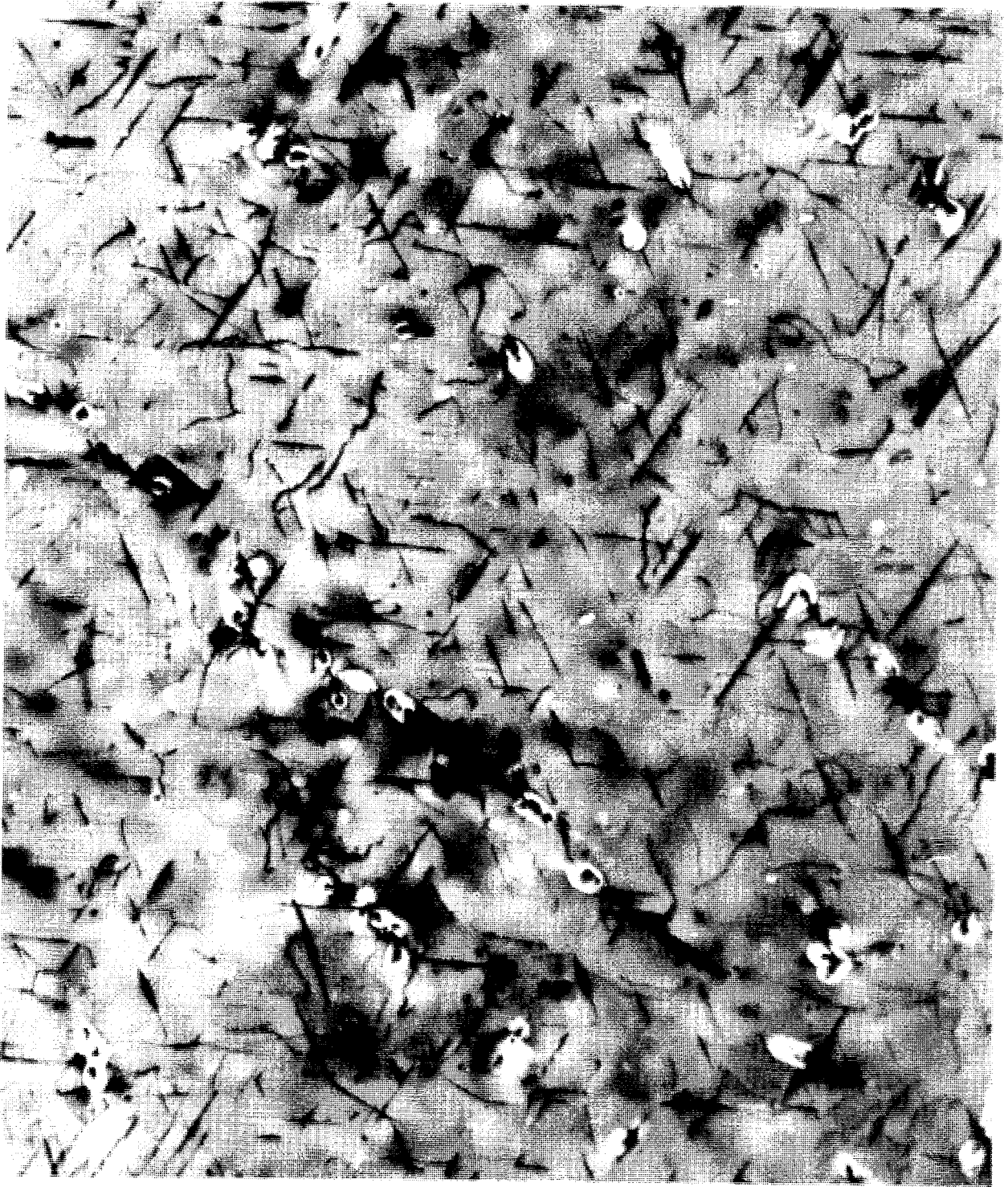
FIGURE 56. Bright Field Micrograph of Solution Treated Type 316 Stainless Steel Irradiated in the EBR-II at 900 °F to 0.8 \times 10^{22} n/cm 2 ( E > 0.1 MeV)
