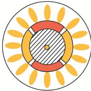
A) Surface Permanent Magnet SPM
