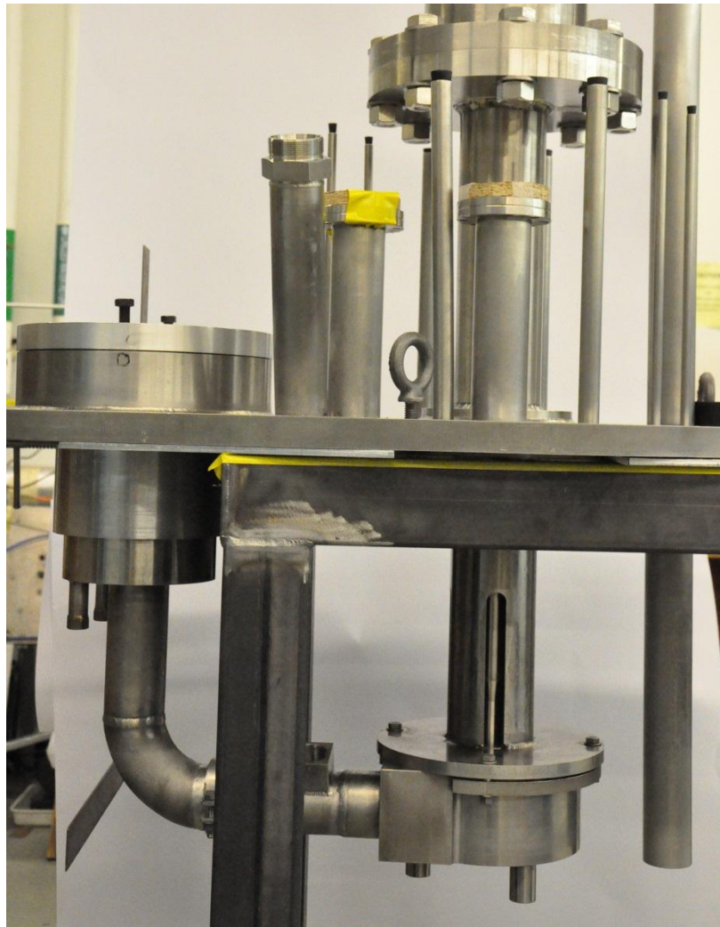
Fig. 5. Sump-style salt pump for inductive-heating loop.
