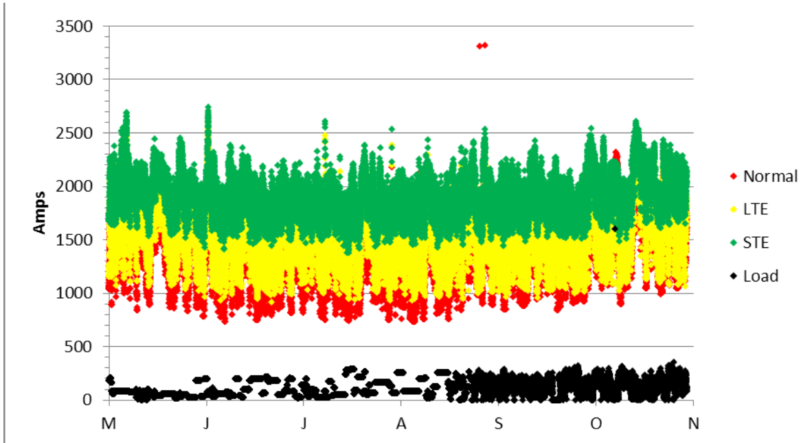
Figure F-6 Overhead line ratings based on Onsite weather station for Site 3 – Summer 2011
