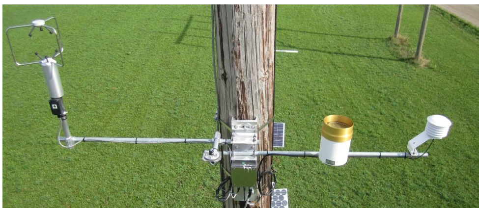
Figure 3-1 Weather station sensor array; anemometer, pyranometer, rain gauge, temperature/humidity sensor (left to right)
