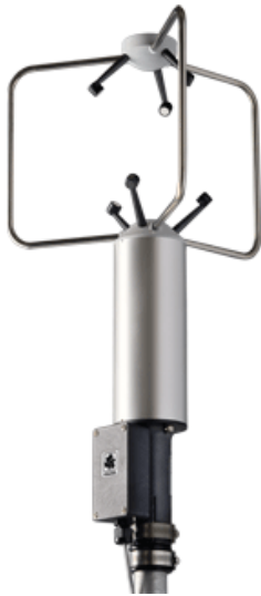
Figure C-8 Three-axis wind speed and direction sensor Note: The wire junction box should always point south. This keeps the wind direction aligned to a known compass heading.
