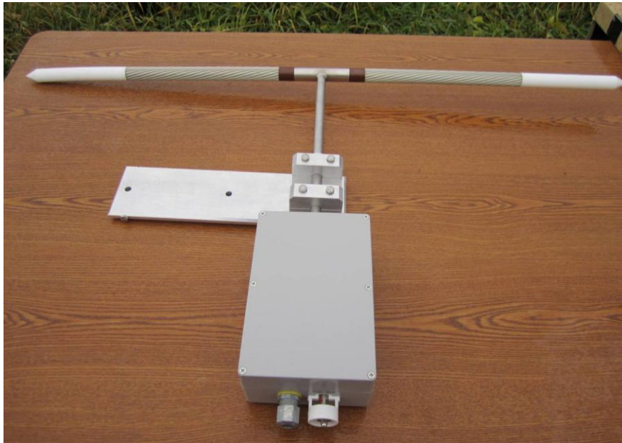
Figure C-56 ThermalRate Sensor Being Readied for Installation
