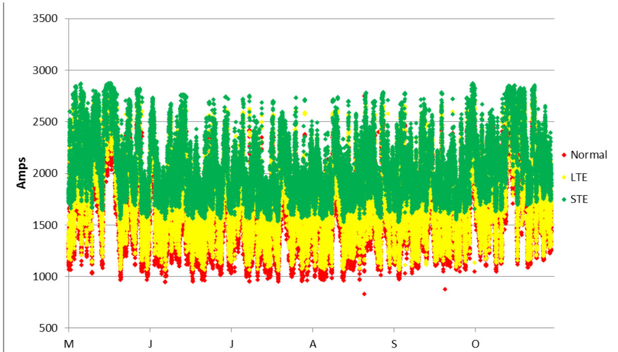
Figure F-42 Overhead line ratings based on ThermalRate device at Site 1 – Summer 2011
