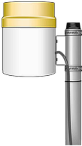
Figure C-7 Tipping bucket rain gauge mounted on an aluminum tube
