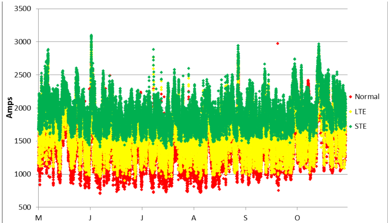
Figure F-44 Overhead line ratings based on the EPRI Sensors at Site 1 – Summer 2011
