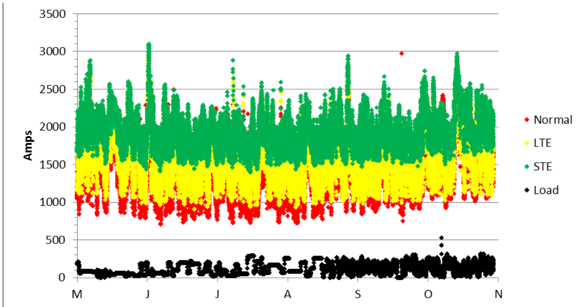
Figure F-9 Overhead line ratings based on the EPRI Sensors for Site 3 – Summer 2
