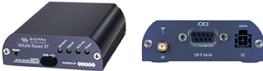
Figure C-28 Isolated front and rear view of Raven XT – This modem is used by the EPRI sensor system
