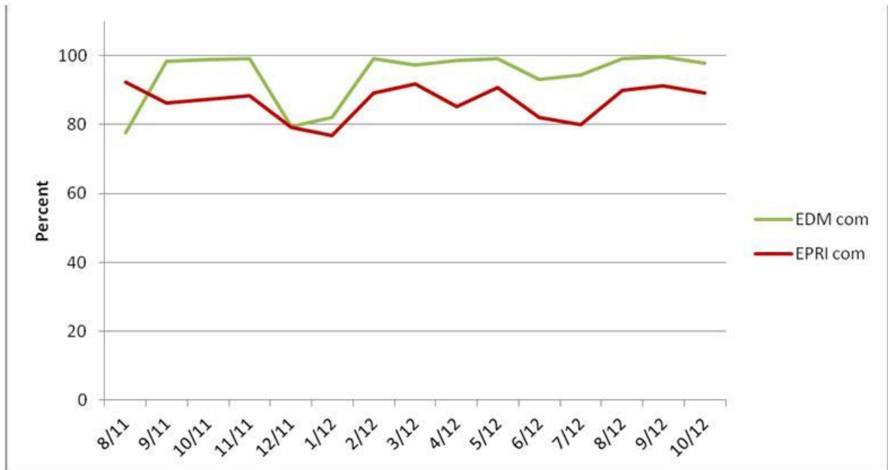
Figure E-7 Communication Availability Between Data Loggers and DTCR Server at Site 1
