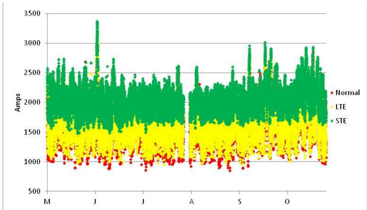
Figure F-52 Overhead line ratings based on EPRI Sensors at Site 1– Summer 2012
