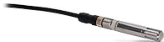
Figure C-5 Temperature sensor removed from housing; temperature and humidity sensors are combined into one unit
