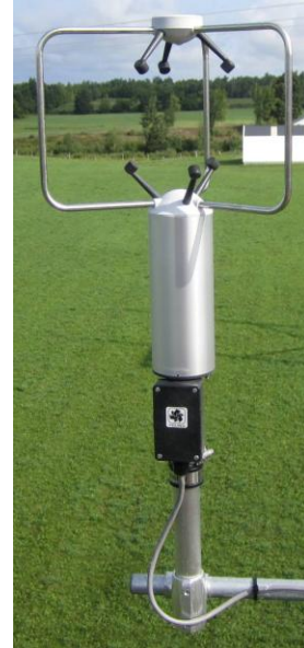
Figure C-8 Three-axis wind speed and direction sensor Note: The wire junction box should always point south. This keeps the wind direction aligned to a known compass heading.
