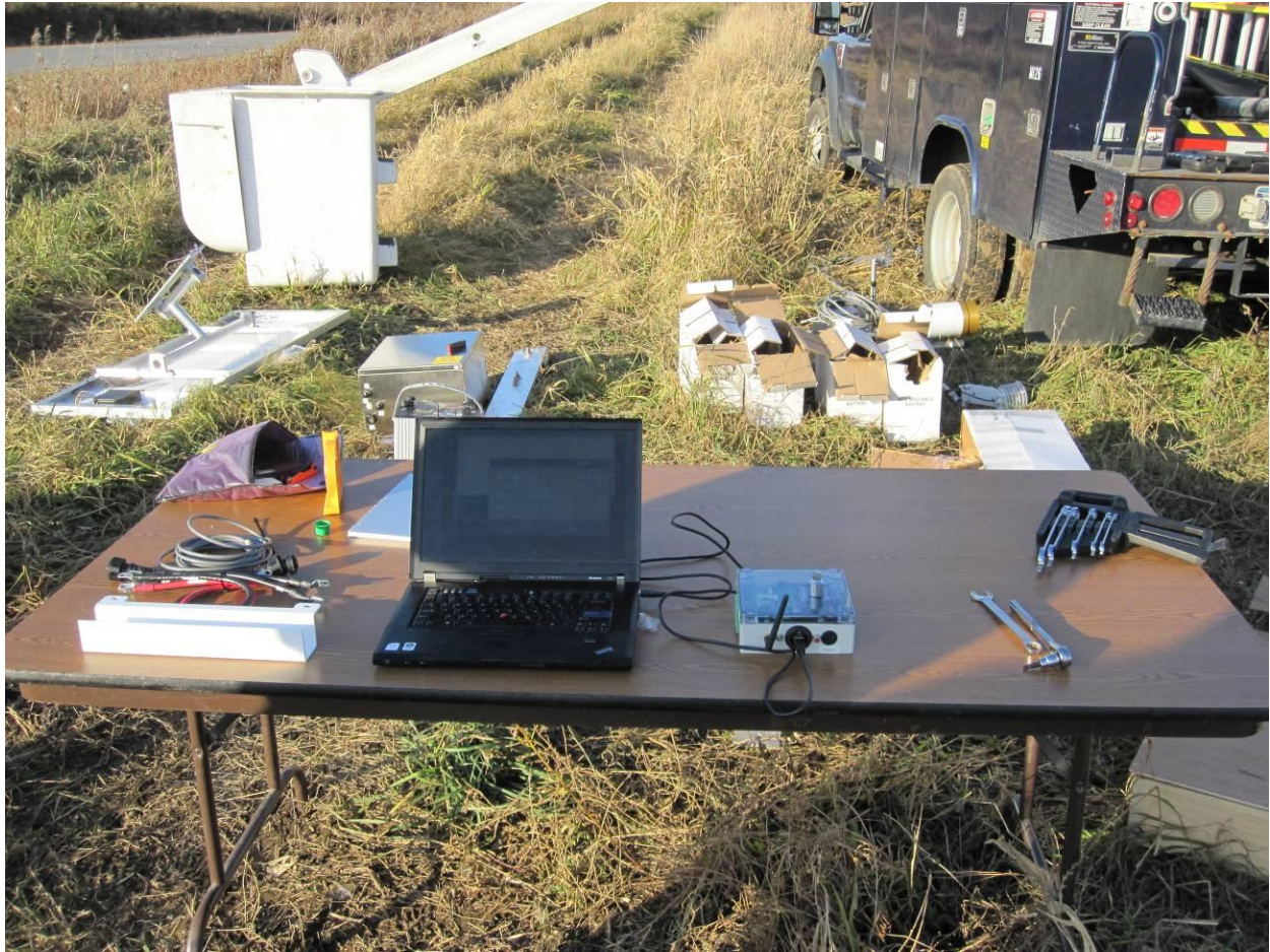
Figure C-43 Remote ZAP Unit used to check communications of the EPRI Sensors in the field
