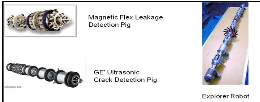
Figure 3-4. Examples of Intelligent Mobile Sensing Devices
