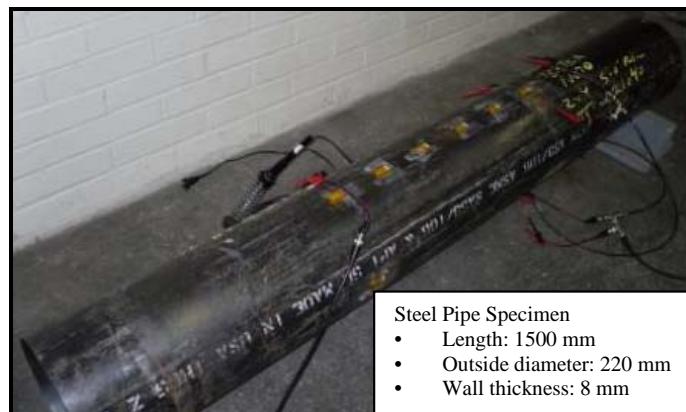
Figure 3-17. Laboratory Transducer Experiment
