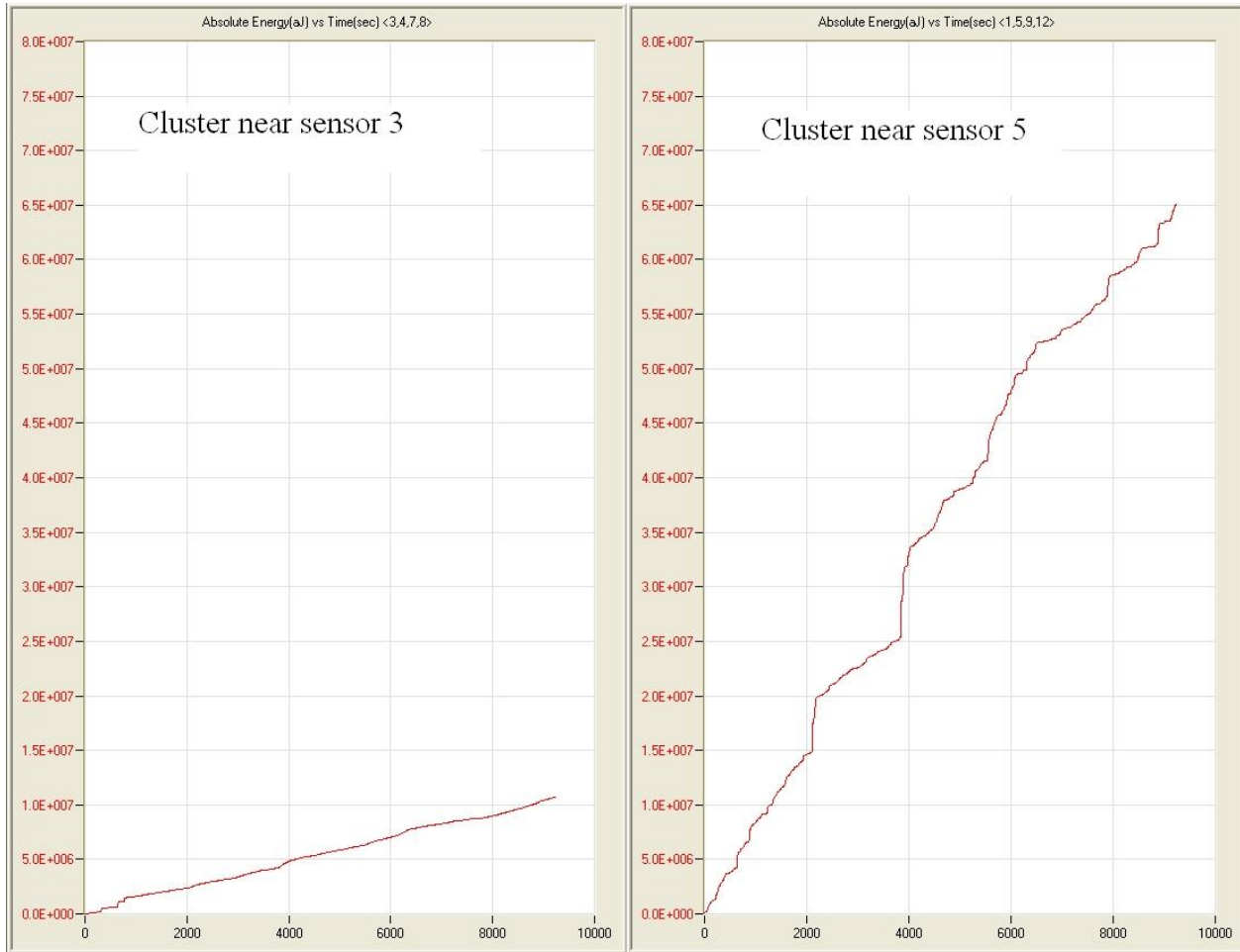
Figure 7-4. Total Absolute Energy as a function of time for clusters near sensor 3 (left, a) and sensor 5 (right, b) for data seen in Figure 7-2.
