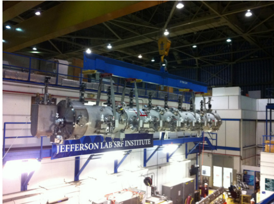
Figure 4: C100 leaving the assembly building.
