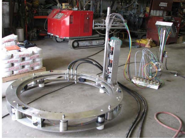
Fig. 3. Cutting tool utilized to cut the tank dome.
