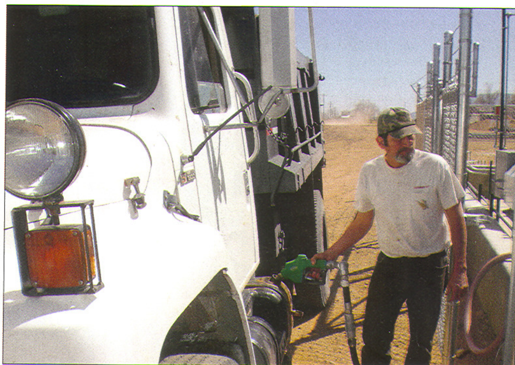
County worker Dave Guerra fuels a dump truck with B40. At present the biodiesel fuel produced at the plant is utilized in the county’s diesel vehicles.
