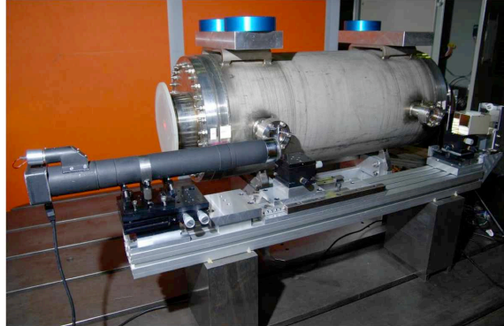
Figure 6. IHEP tank with autocollimator.
