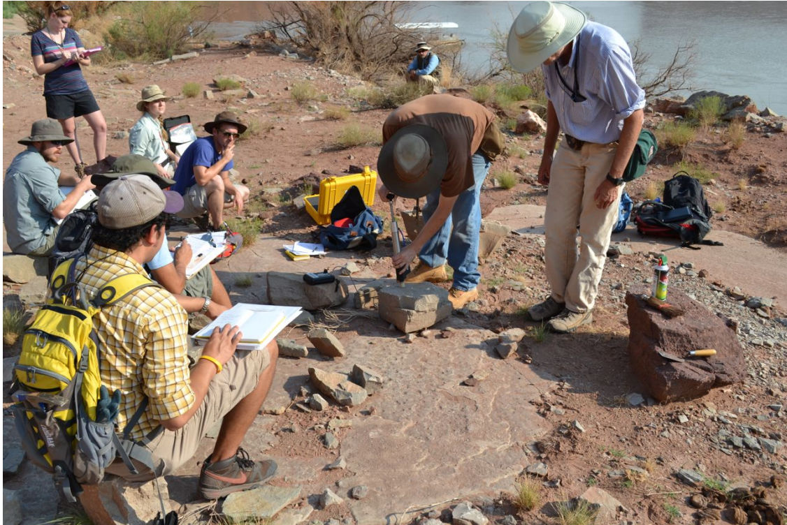
Figure 2. A student uses a field minipermeameter to measure the permeability of a block of limestone in a quarry near the Colorado River.
