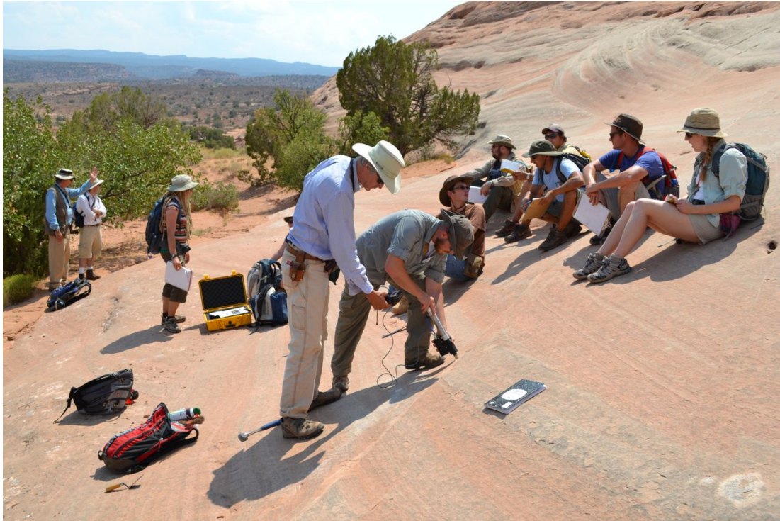
Figure 3. A student measures the permeability of amalgamated deformation bands in the Entrada Formation.
