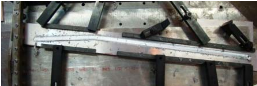
Figure 4.2.2.2.3-13. Photograph of the Completely Welded Subtended Article Showing the Clamping Approach for the Layer 2 and Layer 3 Welds.
