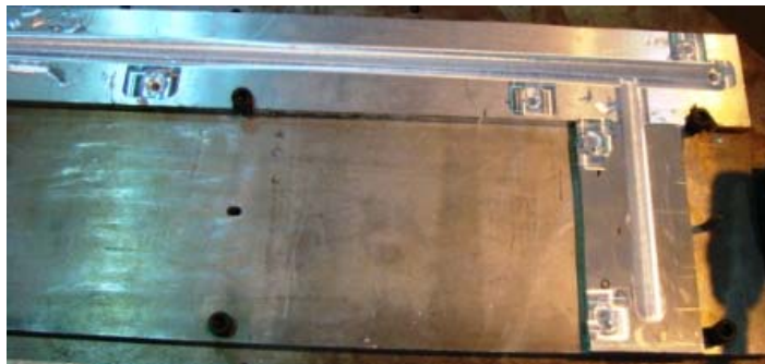
Figure 4.2.2.2.3-11. A Photograph Showing Weld 2 of Layer 1 After Removal of the Welding Flash.
