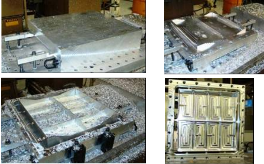
Figure 4.2.2.1-8. Progression of the Machining Operations Reducing a Thick Plate into the Pseudo Bulkhead.
