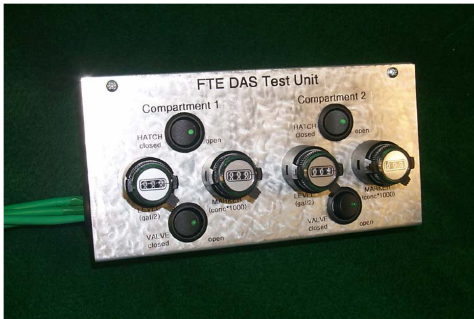
Fig. 82. FTE sensor simulation unit.
