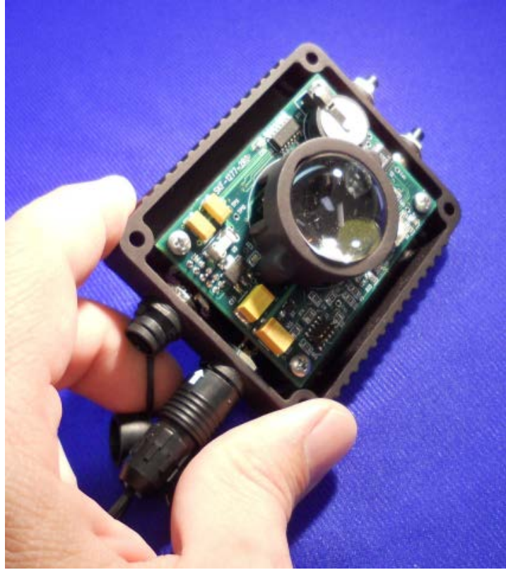
Fig. 43. Marker sensor internal electronics.
