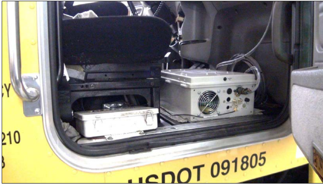
Fig. 91. DAS installed in test vehicle.
