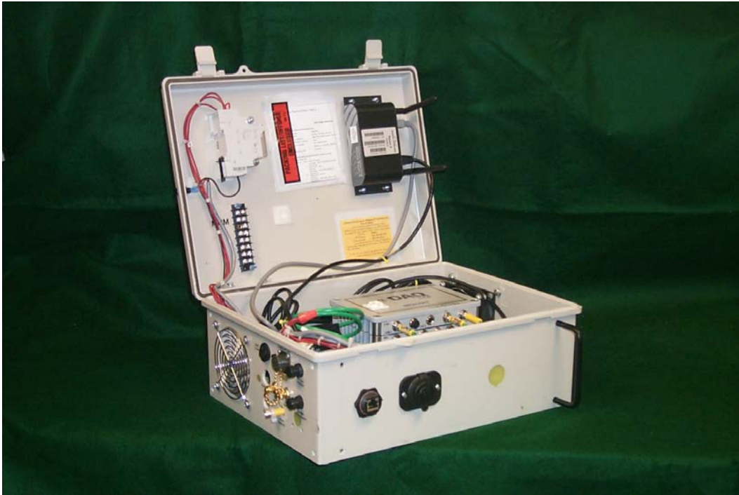
Fig. 49. ORNL DAS used for data collection.
