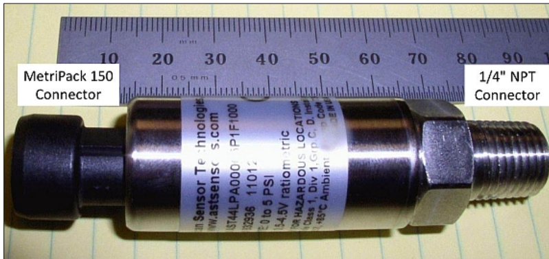
Fig. 32. Pressure-based level sensor used for POC testing.
