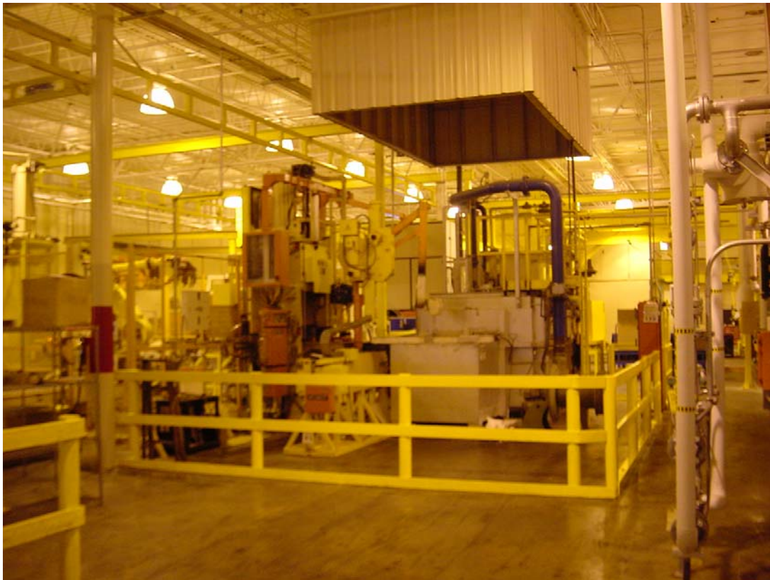
Fig 6 – Rotor die casting manufacturing cell
