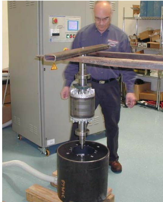
Fig 11 – Magnetization of a prototype rotor
