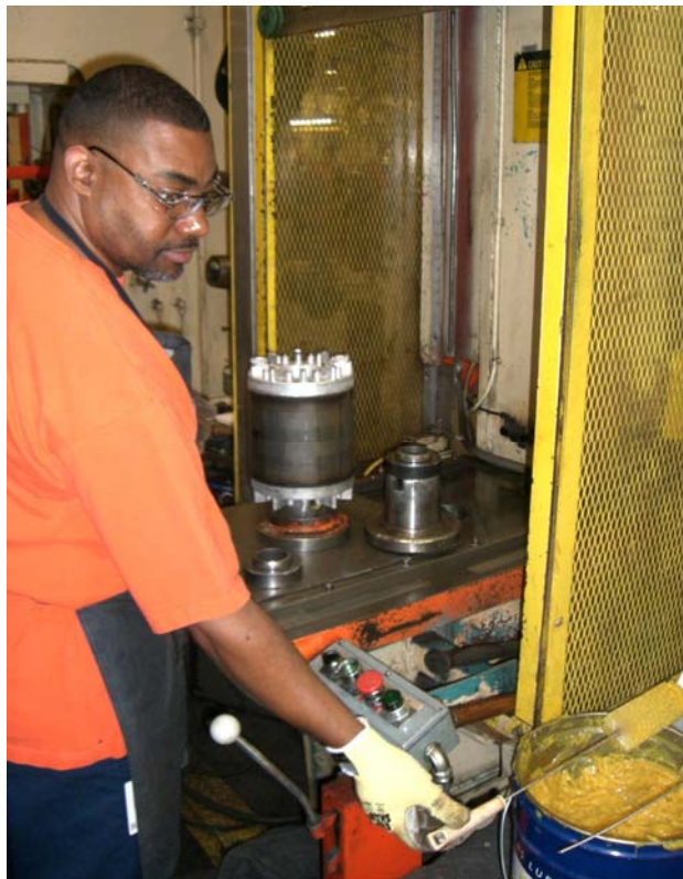
Fig 8 - Shaft insertion following die casting of rotor
