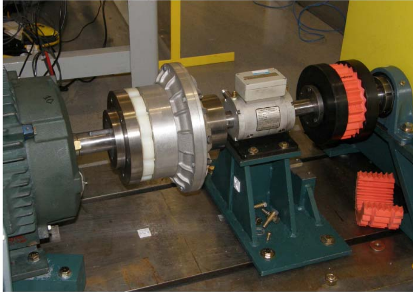
Fig 28 – Soft-Start coupling used to enable synchronization of high torque or high inertia loads
