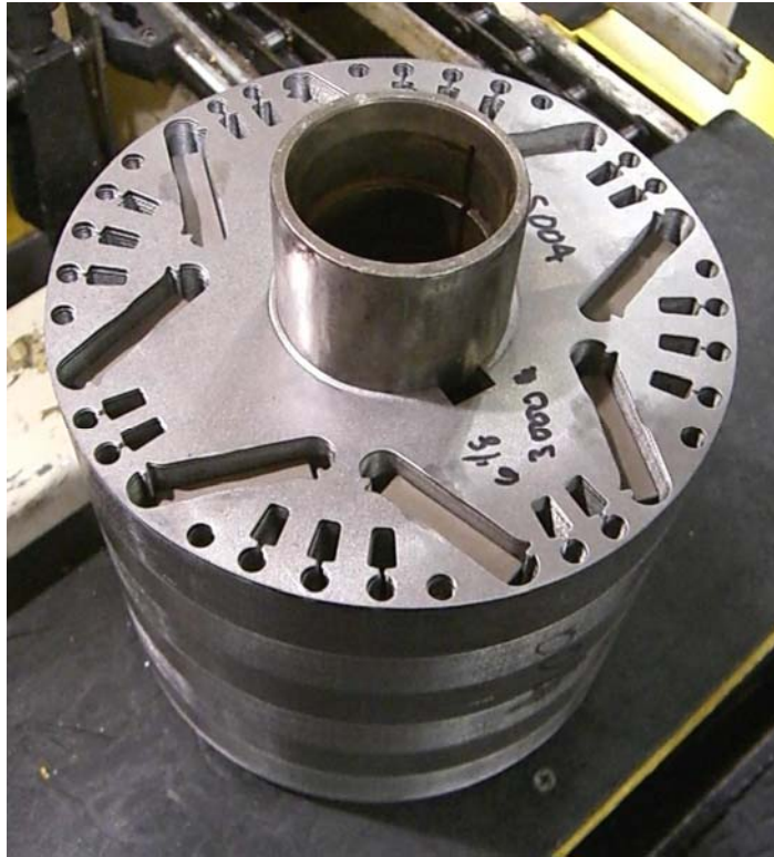
Fig 7 – Rotor core stacked with magnets ready for die casting
